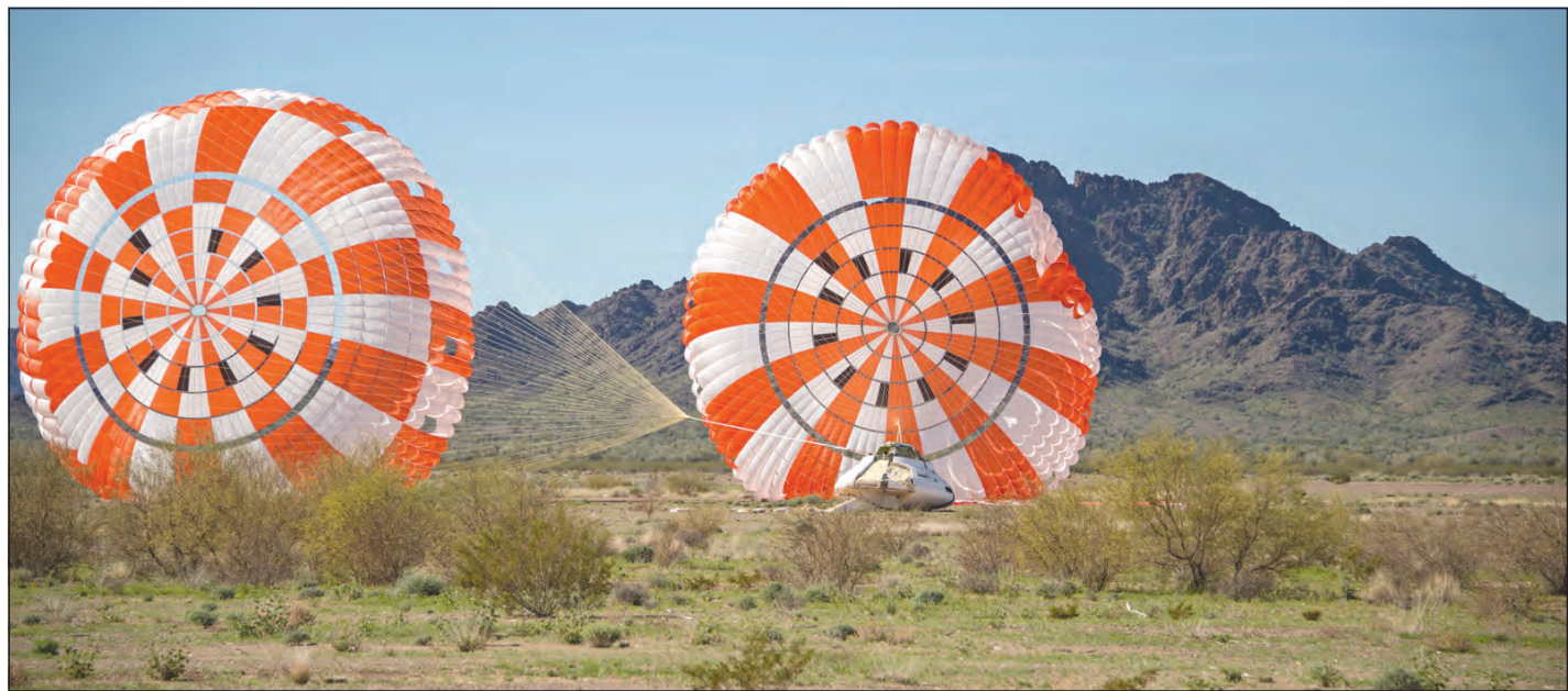
Each of the system’s three main parachutes have canopies made with 10,000 square feet of broadcloth nylon, and risers made of Kevlar, the strong synthetic fiber used in body armor. (US Army photo)
