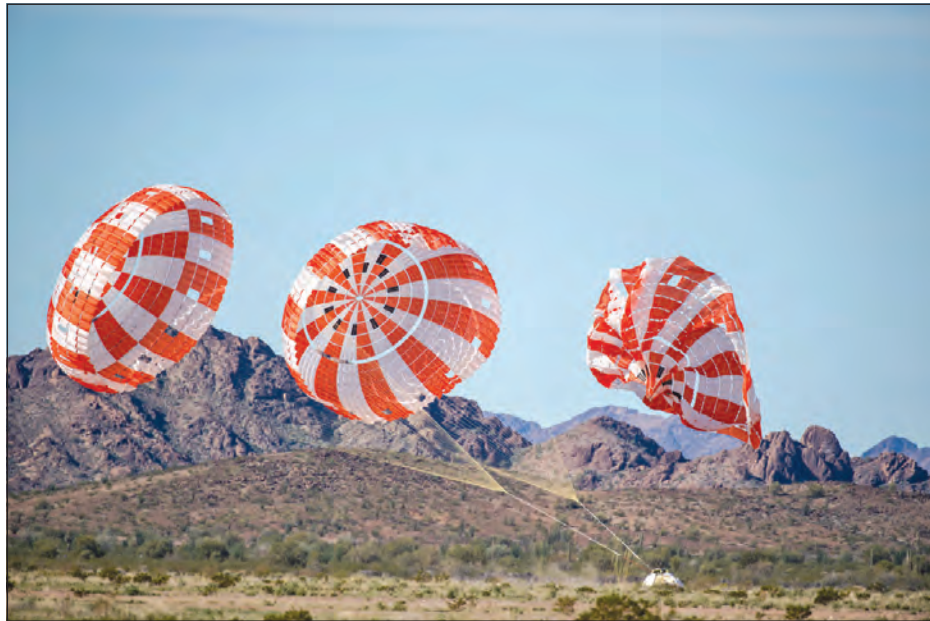
YPG recently completed the second of eight planned evaluation tests of the Capsule Parachute Assembly System on the Orion Space Capsule. With the capsule's first manned flight as little as two years away, NASA hopes to return to the moon, using the lunar surface as both a training and launching site for an eventual Mars mission. (US Army photo)
