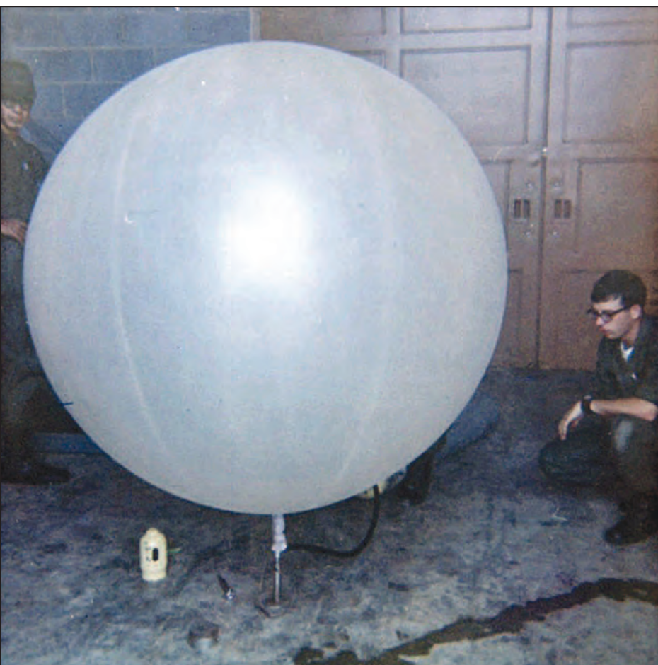
Spc. Stephen F. Mason (right) learns to fill a weather balloon while serving on YPG's meteorology team in 1970. Run by a small team of civilians today, in past decades the team was staffed by dozens of Soldiers collecting weather data. (Loaned photo)
