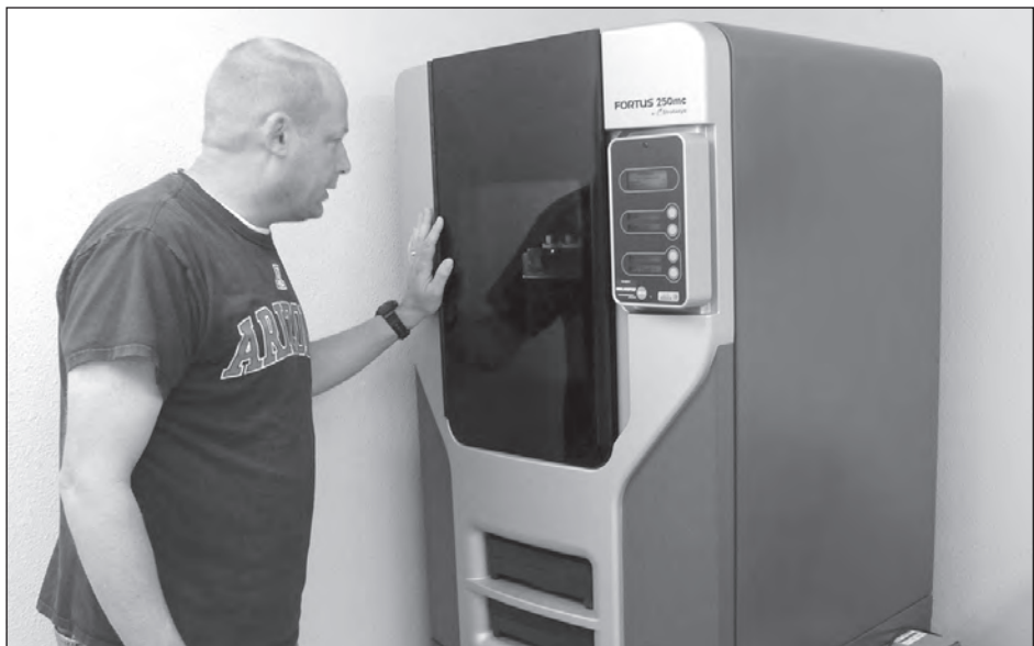
EOM lead Steve Taylor waits for a three dimensional printer to finish a part. The machine, which prints out computer aided design products with an automated, additive process, melts plastic in various thicknesses to produce a part. (Photos by Mark Schauer)
