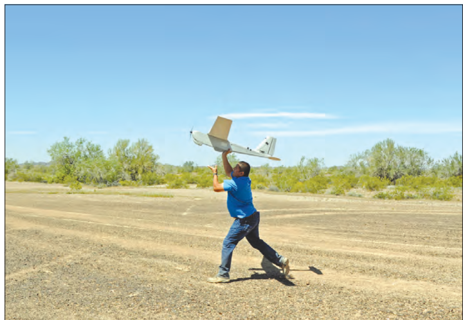
The carbon-fiber propeller spins at about 5,000 revolutions per minute, but, lacking landing gears, the Puma needs an assist from a strong arm to get airborne.
