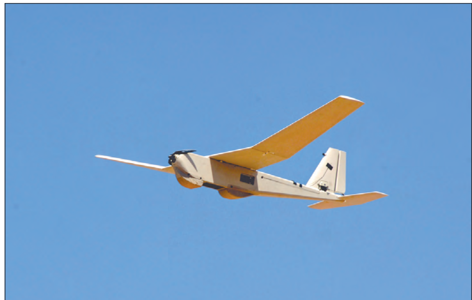
The RQ-20A sprints at over 50 miles per hour, but normally operates at half that speed. Its lithium ion battery, the heaviest component aboard the airframe, powers it for about two hours of flight.
