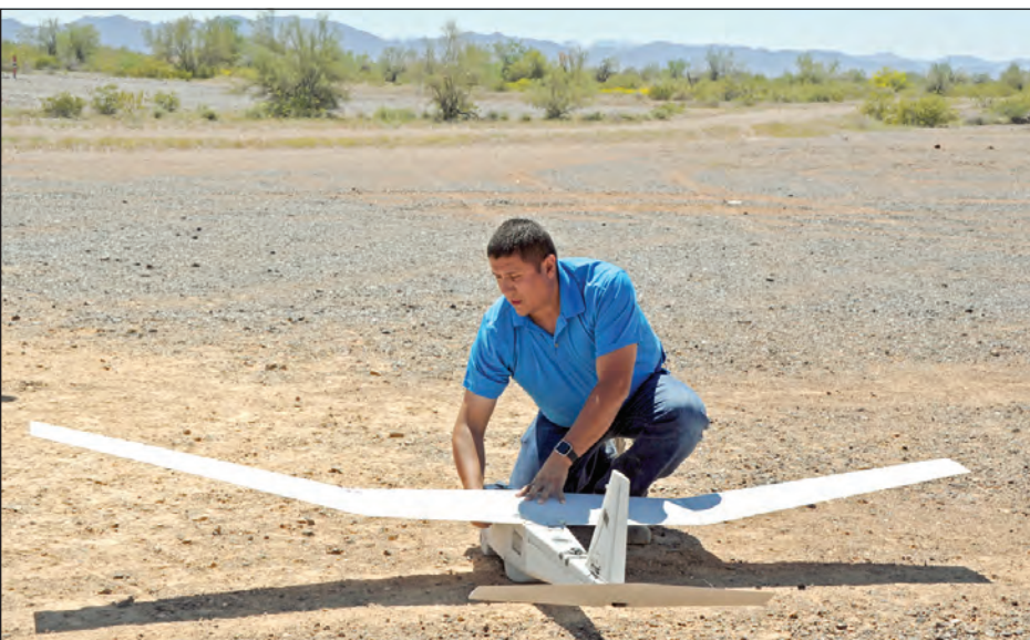
Tipping the scales at under 15 pounds, the RQ-20A can be assembled and hand-launched by a single individual.
