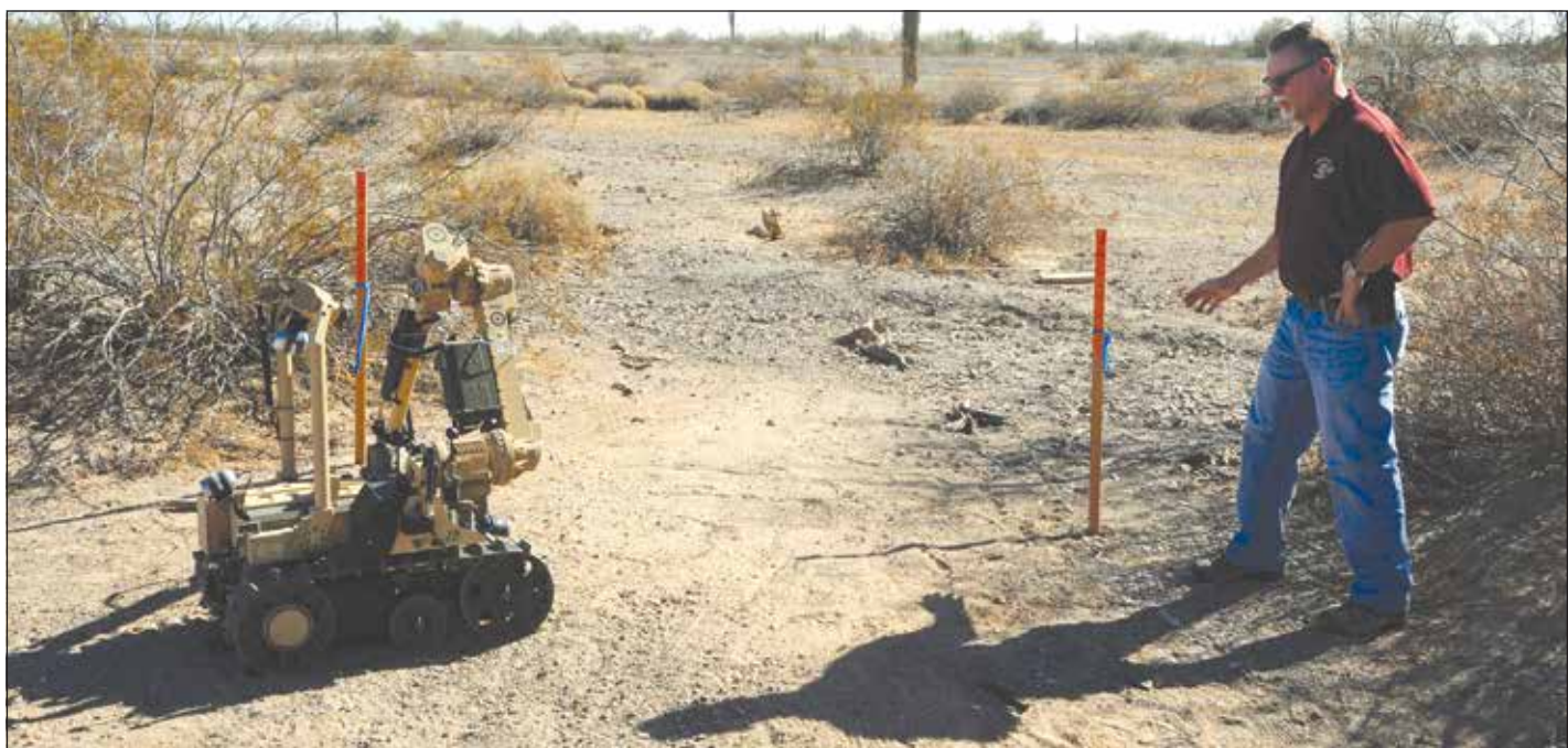
YPG test officer Robert Archibale prepares for a test run of the Standoff Robotic Explosive Hazard Detection System (SREHD), an explosive detecting semi-autonomous system that not only detects things like land mines and improvised explosive devices, but also neutralizes them. Over 400 updates were incorporated into the system after its last test at YPG earlier this year. (Photo by Mark Schauer)
