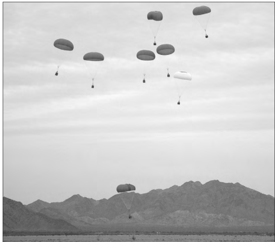
An aircraft dropping EHLSCDS bundles flies in much faster and at a lower altitude than in typical airdrops. In theater, that means cargo planes are in a threat zone for a much shorter period of time and less dispersion which makes it easier for the dropped supplies to be safely recovered before an enemy can respond.
