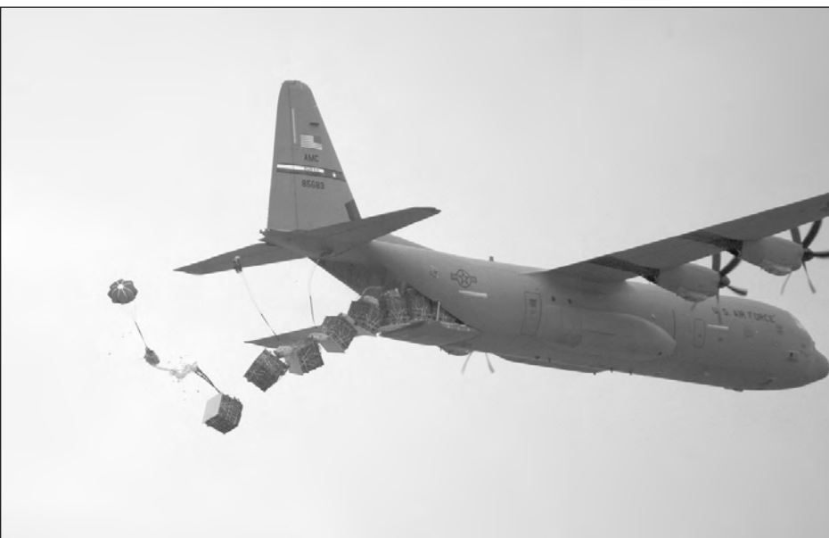
While the EHLSCDS means a tighter-patterned drop once the materials are out of the plane, dramatically greater force is exerted on the bundles when first extracted. YPG testers have been gathering data on the effects of this extraction force on bundles of water bottles, as well as simulated loads of ammunition cans filled with sand and filled water barrels. (US Army photos)
