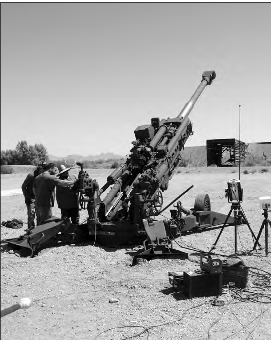
Project Manager Towed Artillery Systems and the U.S. Army Armament Research, Development and Engineering Center are increasing the range of the M777A2 howitzer. The ultimate goal of the program is to demonstrate a maximum range of 70 kilometers while minimizing the cost and modifications to the weapon platform. (Photo by Chuck Wullenjohn)
