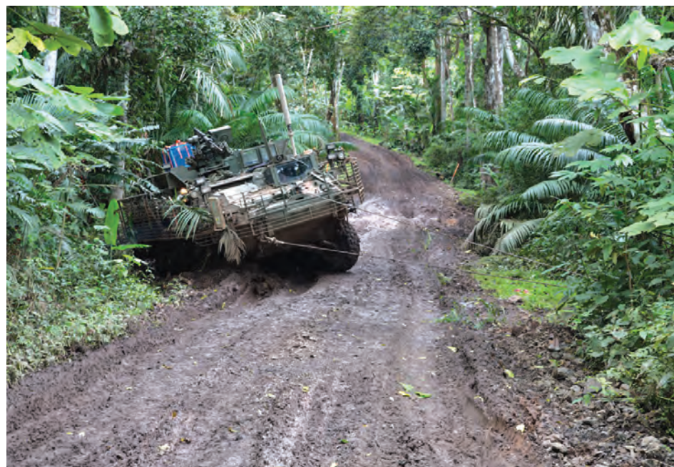
When the vehicle got bogged down by slick, gripping mud that was formerly a road, testers first attempted to extricate it with a single-line pull utilizing the vehicle’s built-in recovery winch. “We do a lot of data collection when it happens,” said Silva. “We try to characterize the terrain, how the vehicle ended up, and the angles of the winch line.” (Photo by Carlos Mora)
