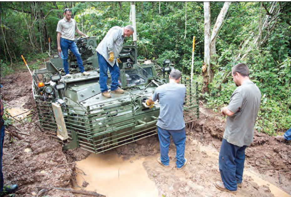
As the rainy season progressed, some roads became too-saturated to support the Stryker's weight and were shut down. "We wanted to make sure we weren't just down here getting stuck," said Omar Silva, test officer. "That's not the goal of the test." (Photo by Carlos Mora)
