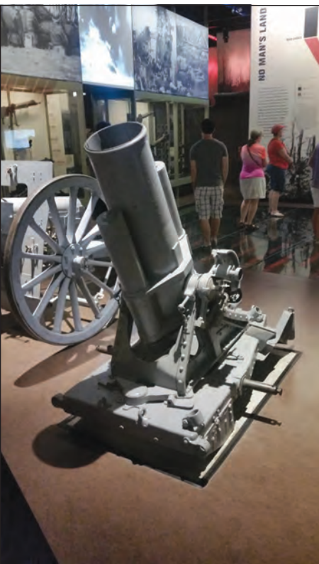
This German 24.5 centimeter heavy trench mortar weighs over 1,600 pounds and had a range of over 3,000 feet. The Germans favored mortars for their economy in both manufacturing costs and use of powder. (Photo by Mark Schauer)
