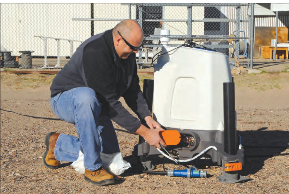
Mark Hendrickson, YPG meteorologist, readies the met team's new man-portable Light Imaging, Detection and Ranging (LIDAR) system that uses a laser to measure wind speeds as high as 600 feet in the air. Once successfully tested, the system will replace anemometers attached to aging towers downrange. (Photos by Mark Schauer)
