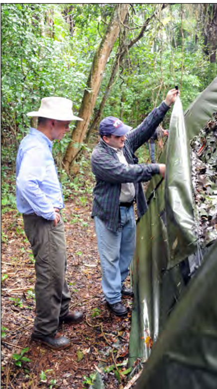
Test officer Julio Villegas (right) shows Army Test and Evaluation Command commander Maj. Gen. Daniel Karbler an airbeam shelter undergoing a long-term exposure test at U.S. Army Tropic Regions Test Center. The tent has no metal frame or poles, relying instead on load-bearing inflatable beams made of a strong fabric compound. (Photos by Mark Schauer)
