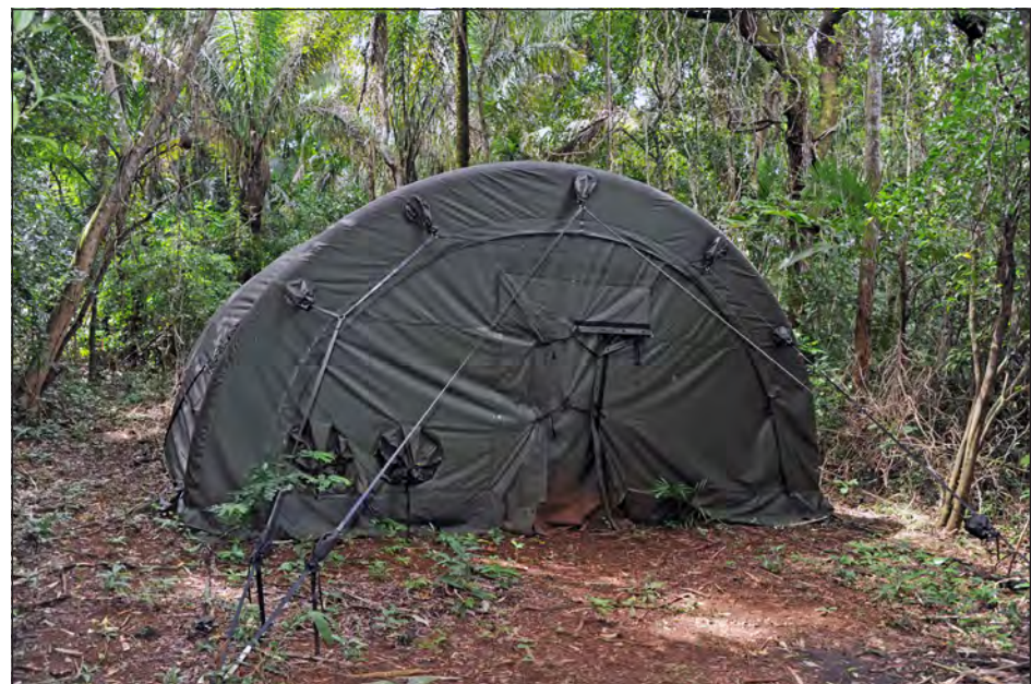
In a harsh jungle, even the tiny failure of a seam could allow moisture into a tent, followed quickly by mold and other microorganisms. "The customer is looking for any kind of degradation of materials caused by biological growth on the material," said Julio Villegas, test officer. "It could be fungi, algae, any kind of biological aggressor."
