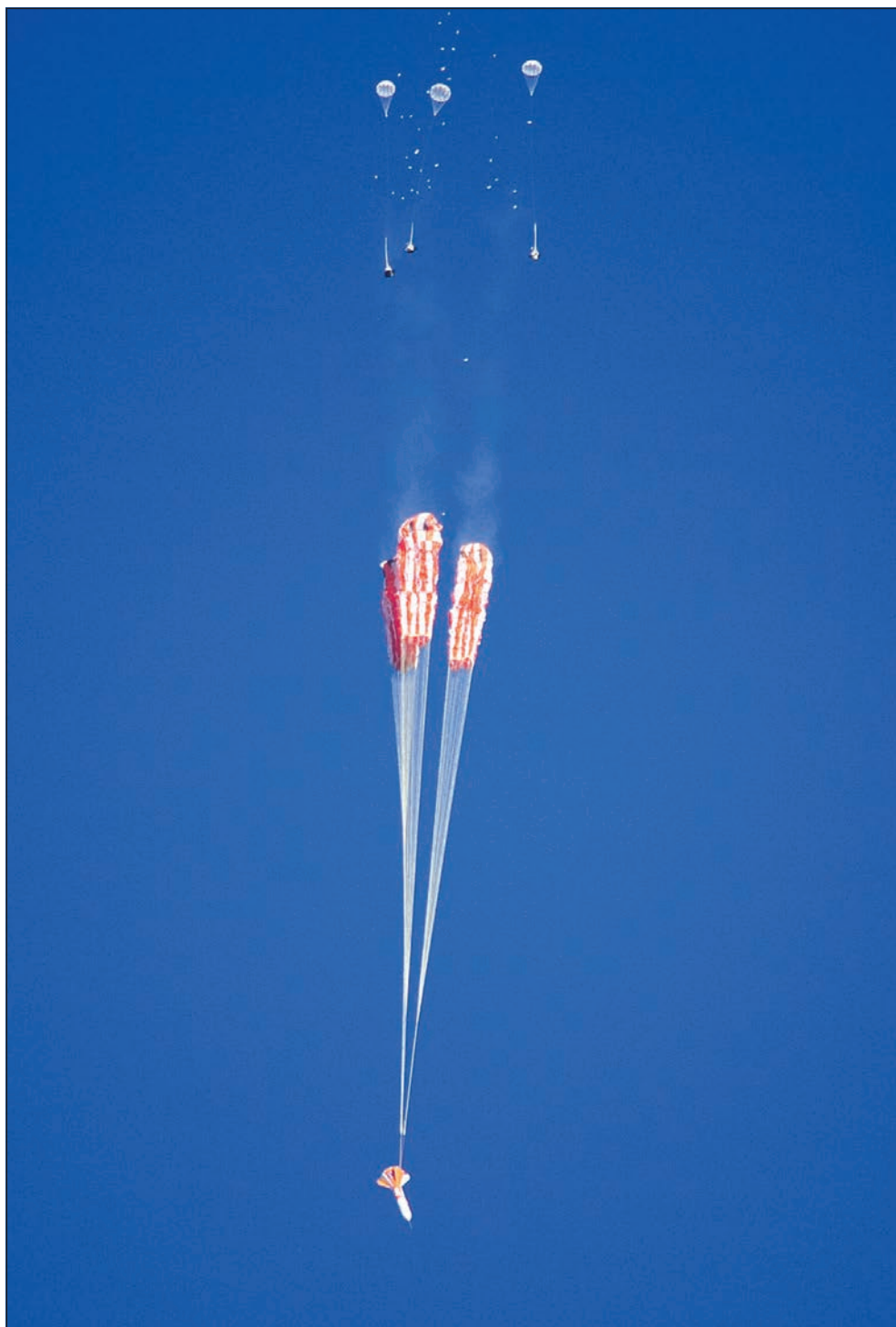
The Capsule Parachute Assembly System (CPAS) for the Orion space capsule underwent its 17th and final developmental test at the proving ground earlier this month. The test used a 44-foot long dart attached to a pallet instead of a mock-up of the Orion capsule. (Loaned photo)
