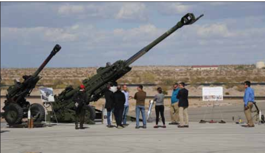
Mike Dickerson, safety engineer in the Ground Combat Test Directorate, highlights the capabilities of the M119 and M777 howitzers, both of which have been tested at YPG for many years. The visitors expressed great interest in the M777’s new chrome tube that significantly extends the life of the barrel.
