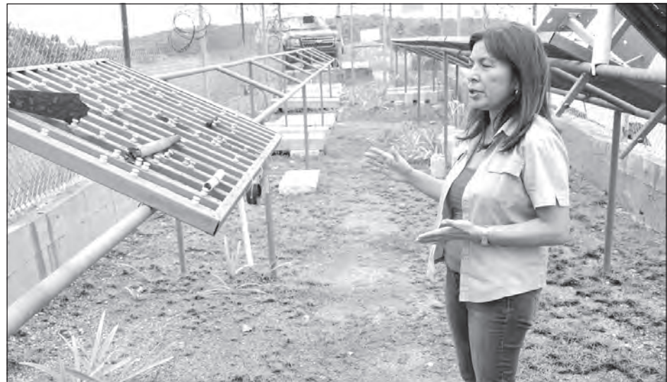
Luisa Wong, test officer, checks on items undergoing testing at Tropic Regions Test Center's breakwater exposure site. TRTC testers expose all manner of equipment in tropical environments, from small samples of paint and metal to uniforms, rucksacks, and weapons. (Photos by Mark Schauer)
