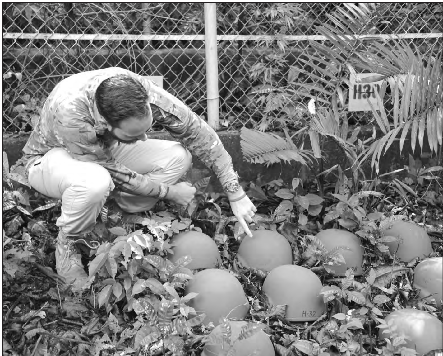
Testers at YPG's Tropic Regions Test Center are conducting an exposure test of the Enhanced Combat Helmet, storing the headgear in ankle-deep leaf and biomass-strewn ground inside a locked double fence cage set within a triple canopy jungle. Here they contend with all the environmental stresses that the jungle can dish out, from high humidity and precipitation to thick mud and vegetation. (Photo by Mark Schauer)
