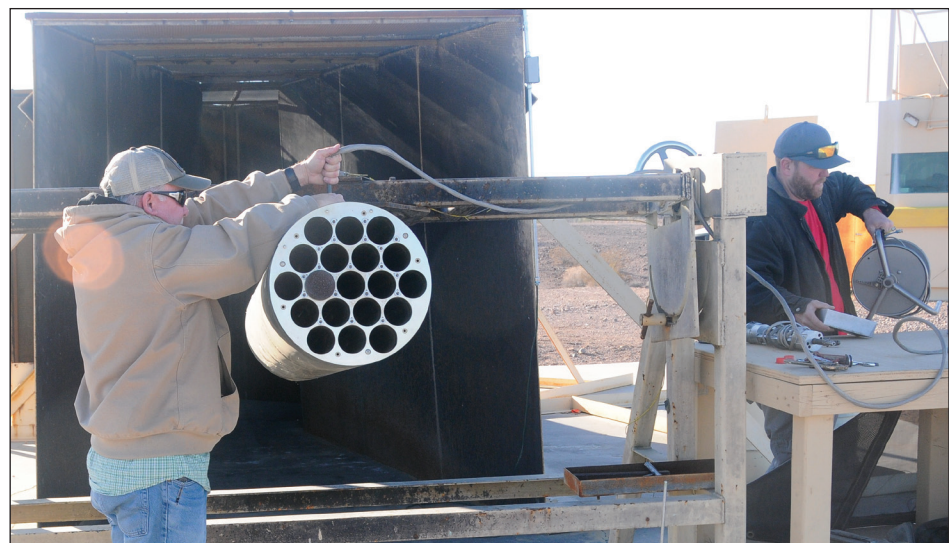
Aircraft armaments lead Dave Gresham (left) and specialist Justin Ferguson prepare a M261 rocket pod for a test fire from a fixed mount at Yuma Proving Ground. Test firing takes place from both fixed-mount gun emplacements on the ground and aboard a flying platform. (Photos by Mark Schauer)
