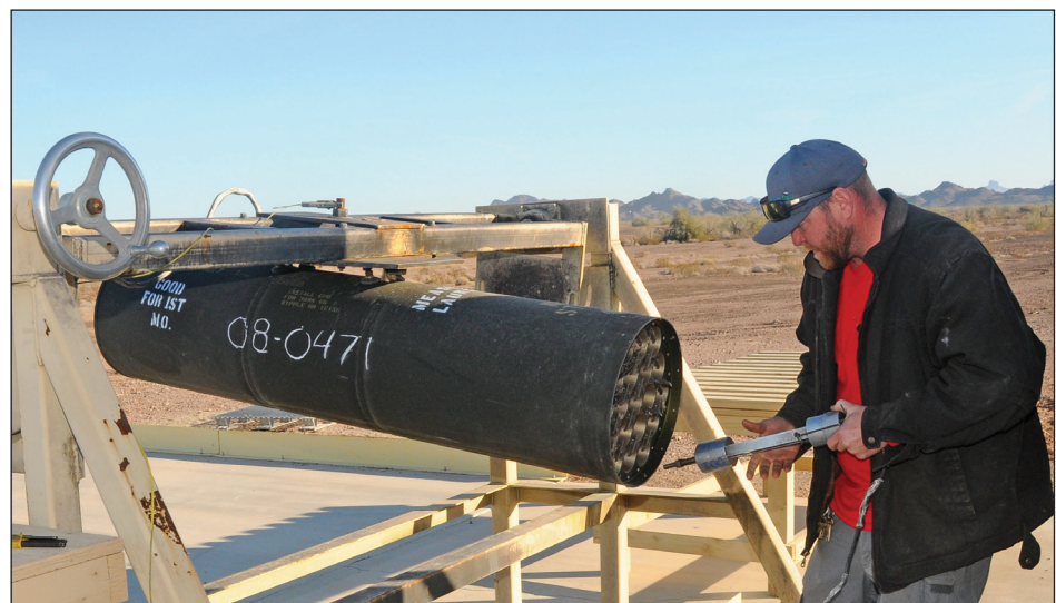
Aircraft armaments specialist Justin Ferguson prepares for a rocket fire from a fixed stand at YPG. Setting up a test site means installing the specialized equipment evaluators use to gather data from a test fire and conducting numerous safety checks to ensure the people and equipment on site come through the inherently dangerous fires unhurt and undamaged.
