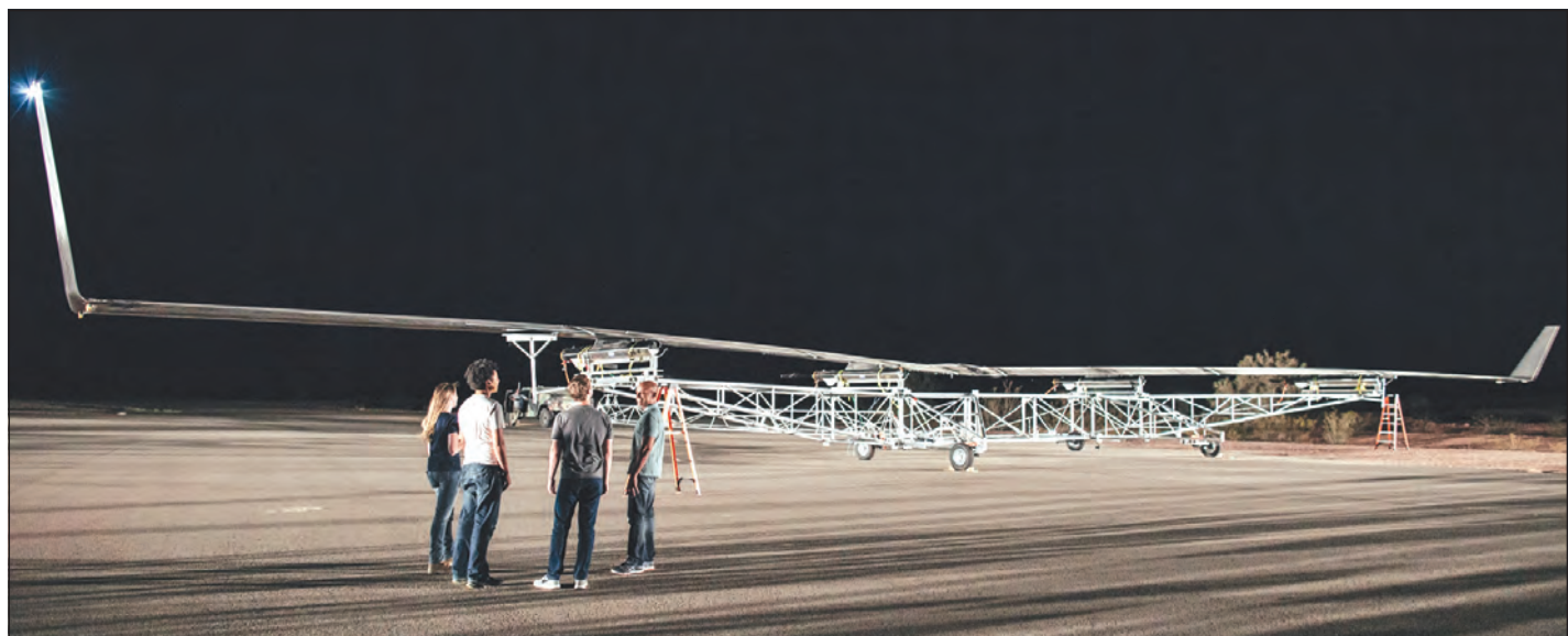
Aquila, Facebook's solar-powered plane, has a wingspan wider than a Boeing 737 but weighs less than even the smallest compact automobile. The unmanned aircraft will carry a communications payload that will use lasers to transfer data more than 10 times faster than existing systems and aim its beams precisely enough to hit a dime more than 11 miles away while in motion.
