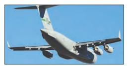
To study the vortices caused by cargo planes, YPG testers conducted more than 150 flights across all hours of the day and night for two weeks, using a LIDAR-equipped chase plane to characterize the aerial disturbance left in the plane's wake. The testers frequently changed their flight approaches in real time to accommodate different wind and weather conditions.
