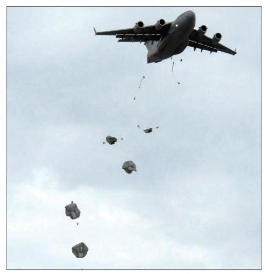
YPG's Air Combat Systems Test Directorate has for several years conducted tests on the C-17 Globemaster to determine the amount of time and distance necessary to safely separate each element of a multi-element insertion of combat parachutists. Data collection techniques developed for this study may have far reaching impacts on how wing tip vortices of both military and commercial aircraft may be studied in the future. (Loaned photos)
