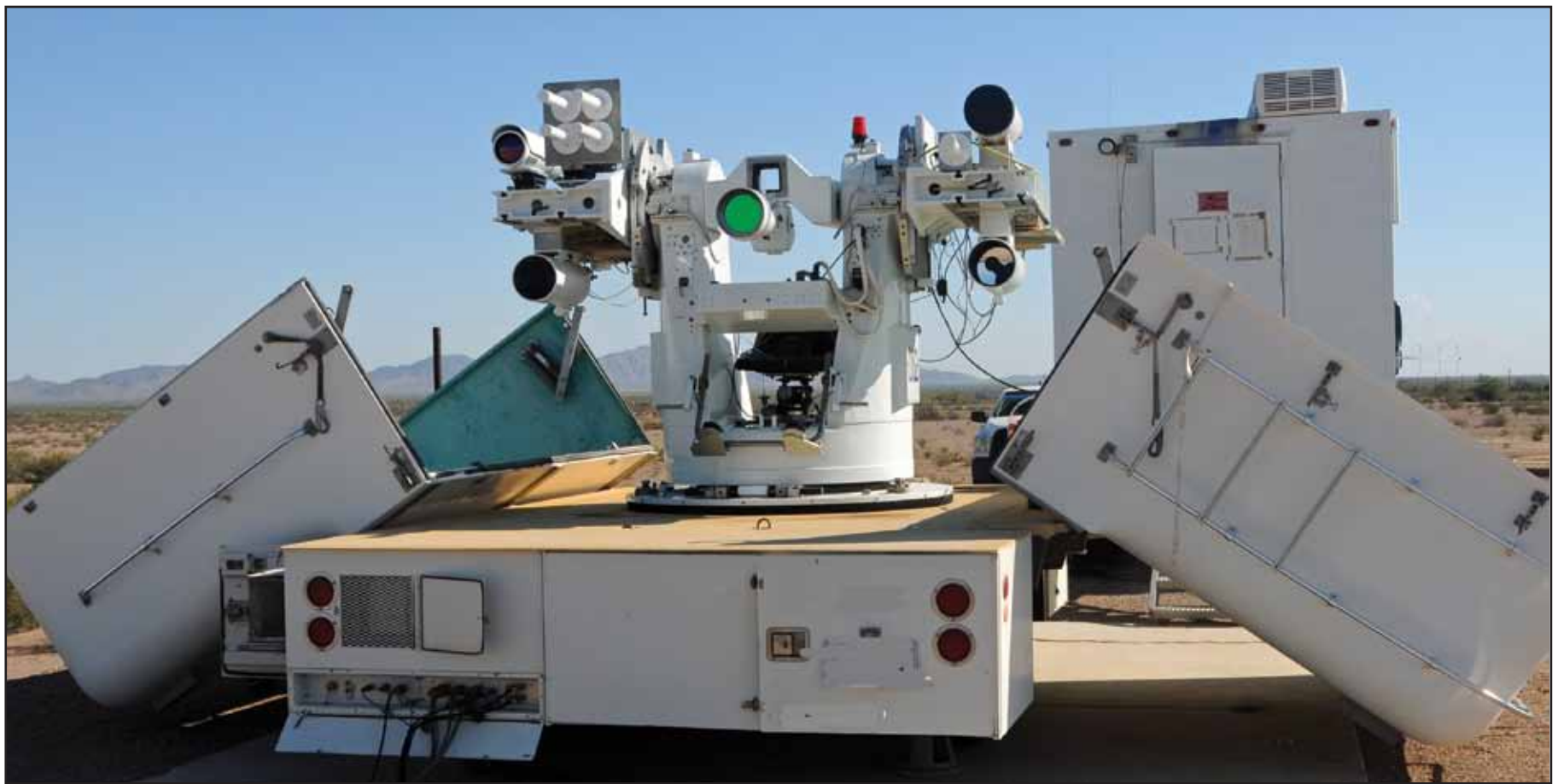
Kineto Tracking Mounts like the one seen here are equipped with multiple cameras, some with lenses as wide as 100 inches, and telemetry devices to capture imagery and other data from artillery and air drop tests. (Photos by Mark Schauer)
