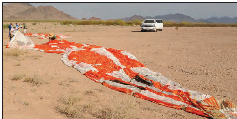
Once the drop was completed, personnel fanned out and carefully recovered the massive deployed parachutes and lines from the desert floor, as seen here. Testers want to evaluate any damage that may have occurred to the parachutes, and know that it was not incurred from the recovery efforts. (Photo by Mark Schauer)
