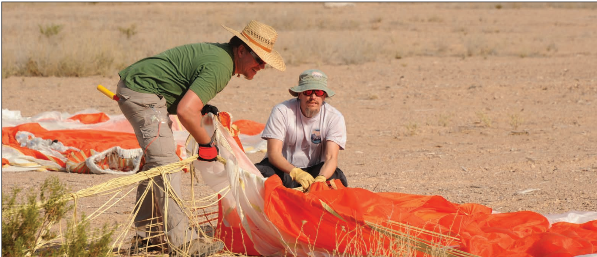
Each of the system's three main parachutes have canopies made with 10,000 square feet of broadcloth nylon, and risers made of Kevlar, the strong synthetic fiber used in body armor. (Photo by Mark Schauer)
