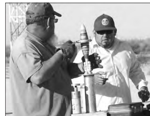
YPG weapons operators John Devine (left) and Daniel Zendejas prepare a M769 full range practice mortar round for a test fire. The inert round, which has the shape and characteristics of the 60-millimeter mortar round commonly used by combat infantrymen, is tested just as rigorously as a live mortar round. (Photos by Mark Schauer)
