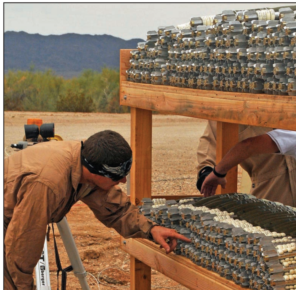
Ready to go: Weapons operator Gerald Miller takes one last look at the 320 mortar rounds he will soon be feeding into a 60mm mortar tube. The test called for an initial rate of fire of 30 rounds per minute for four minutes, or one every two seconds.
