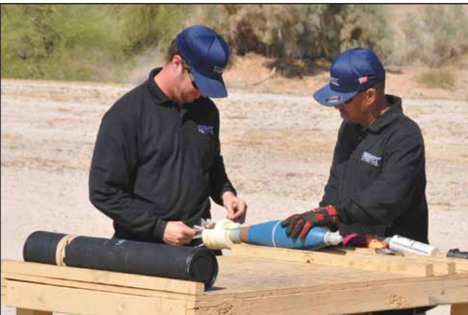
YPG weapons operators Tristan McCollum (left) and John Delgado prepare a 120mm mortar round for a test fire from the prototype mortar ballistic cannon tube under test. Mortar rounds have advanced in recent years with projectiles such as the GPS-guided XM-395 Precision Guided Mortar Munition, yet the tubes they are fired from have remain unchanged for more than two decades.
