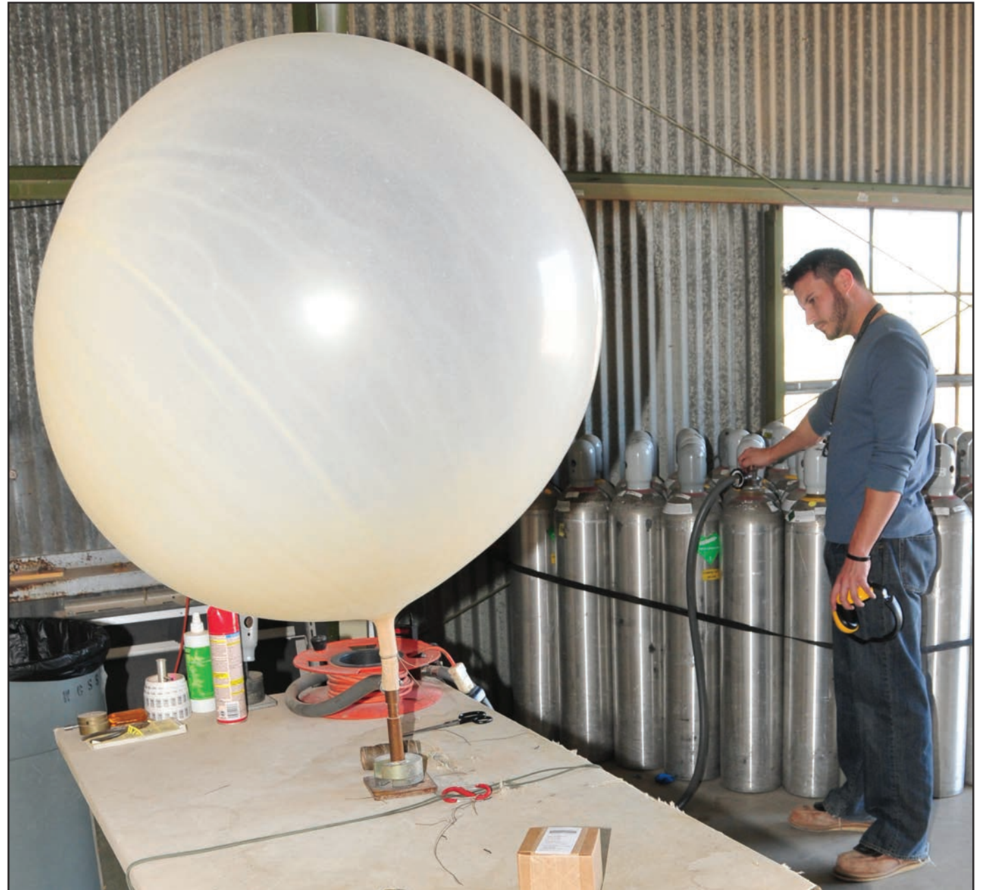
Contractor Daniel Meza fills a standard weather balloon with helium. He is looking at a display next to the cable reel that has the readout of the flow meter. The flow meter indicates how much helium is placed in each balloon.
