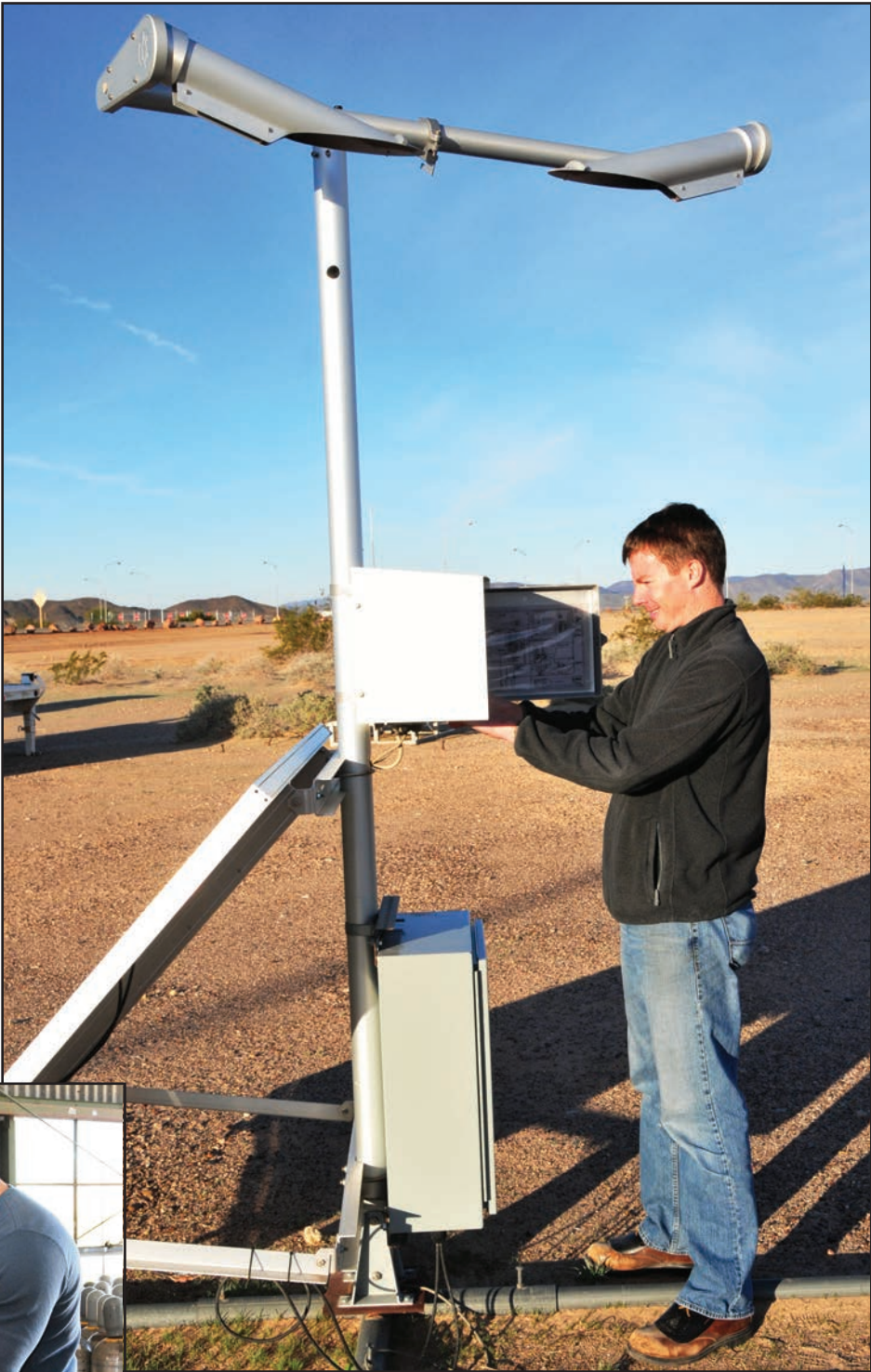
Nickolas McColl (above) verifies the operation of a visibility sensor. This sensor measures how much “stuff” is in the atmosphere and calculates how far one can see. Dust, rain, and fog can reduce visibility, but, normally, YPG experiences nothing but clear skies. Daniel Meza attaches a standard weather balloon to the nozzle of the helium fill station. This is where the balloon is filled just before it is launched with a radiosonde attached to it. The devices measure temperature, humidity, pressure (from which height is calculated), and winds (calculated from GPS data received from the device).
