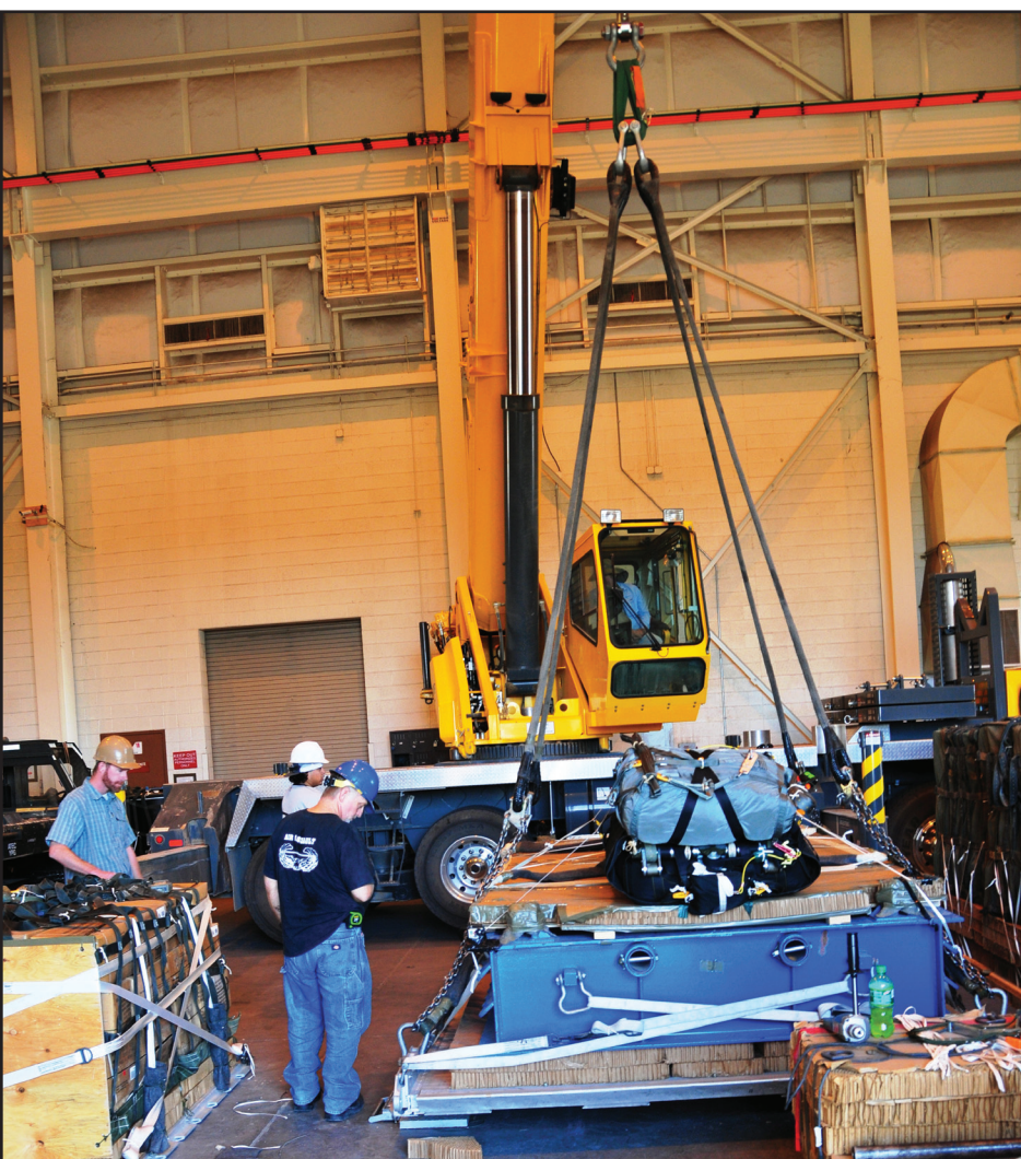
This rigged bundle is ready to be loaded onto a K-Loader, visible in the background, along with other bundles. From here, the heavy loads are driven to the aircraft and loaded aboard.
