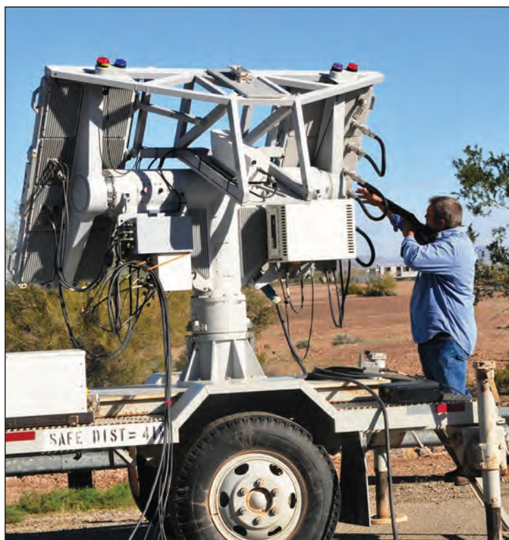
Justin Keesey from the radar section, demonstrates the power of a tracking radar by tracking a .177 caliber BB.
