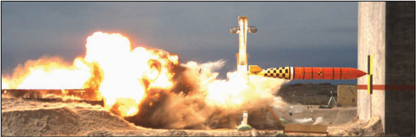
The Legacy Warhead Improvement Program testing 2,000 lb. Penetrator Warheads at Holloman High Speed Test Track, N.M. The projectiles were fired at different velocities into various configurations of hardened concrete targets to assess the weapon's survivability. (Photo by HHSTT)
