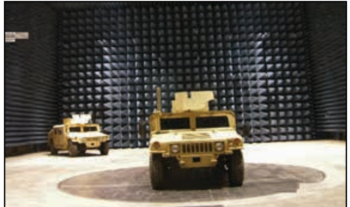
The main test chamber in the Electromagnetic Vulnerability Assessment Facility, which is over 100 feet long, can test everything from computer networks to tanks and small aircraft. (Photo by D. Hamilton)
