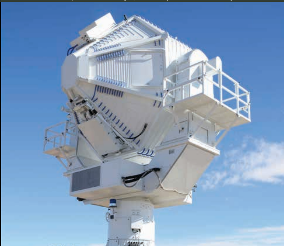
One of three Multiple Object Tracking Radars (MOTR) in use at WSMR. These radars are capable of tracking up to 40 objects simultaneously.
