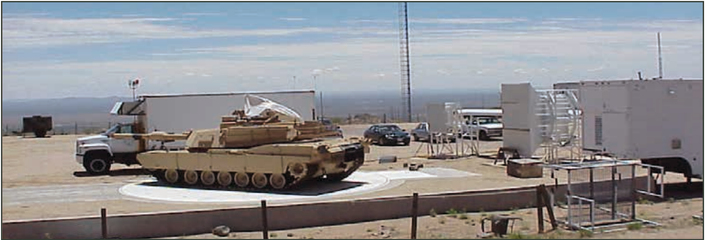
Electromagnetic testing of a tactical unit on SVAD's 80-ton, 33-foot turntable.
