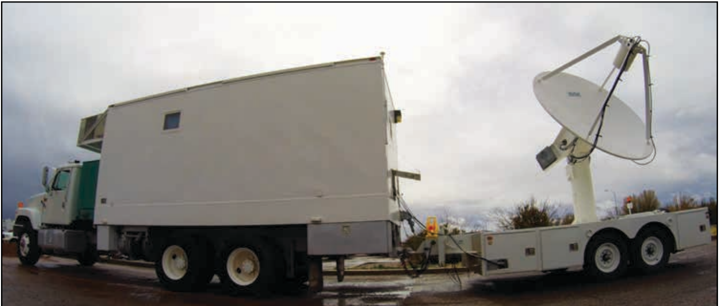
WSMR operates the Transportable Range Augmentation and Control System (TRACS), Transportable Telemetry Systems (TTS) [pictured], and mobile telemetry systems available for mission support, both for on range instrumentation and safari missions. (Photo by G. Palombit)
