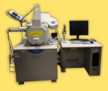
Scanning electron microscope for high-magnification imagery and chemical composition analysis
