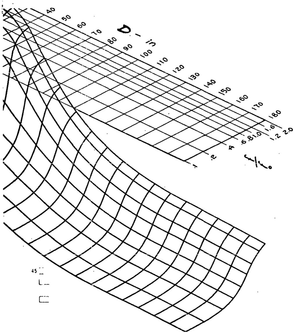
FIGURE 519.2-4. Random vibration prediction surface, low frequency (Cont'd)
