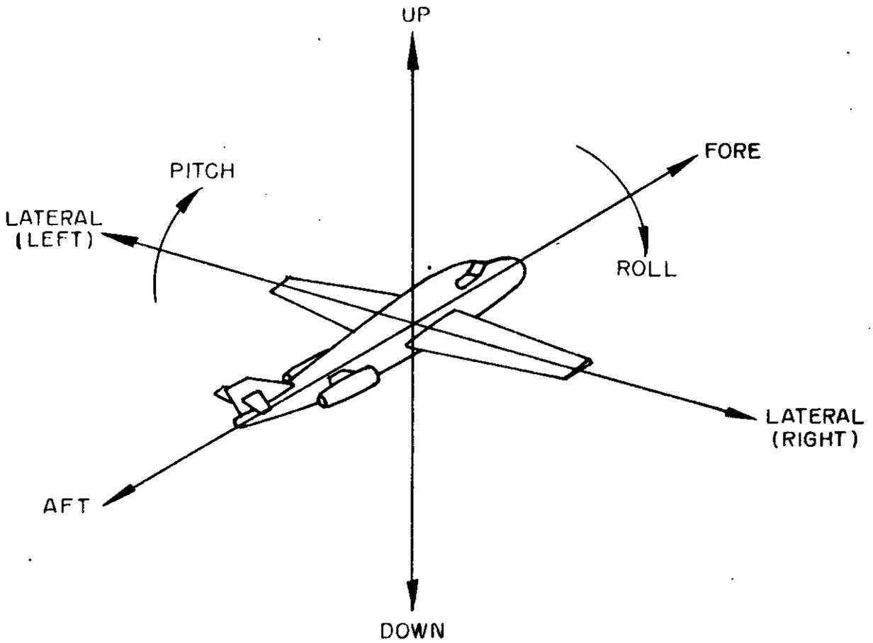
FIGURE 513.2-1. Direction of Vehicle Acceleration
