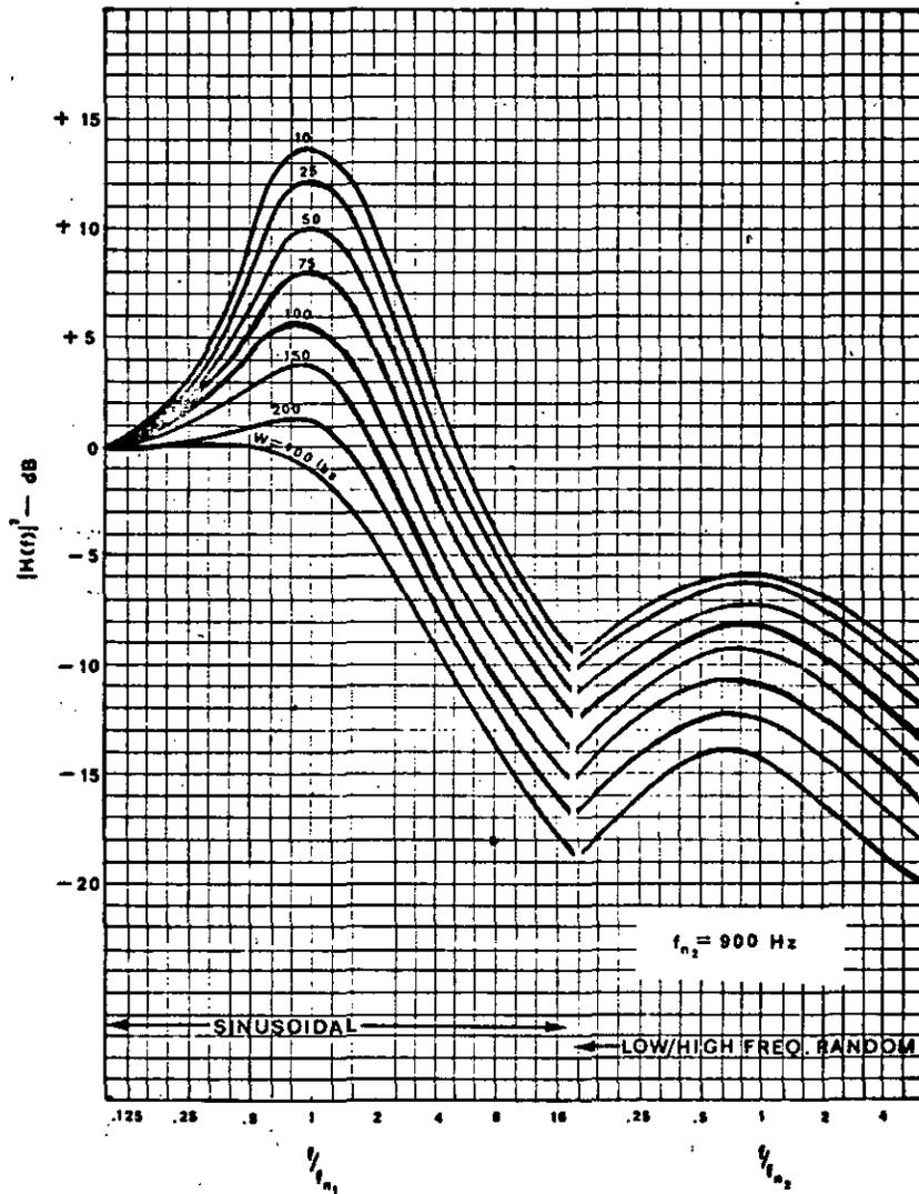
FIGURE 519.2-19 Transfer functions for non-isolated equipments
