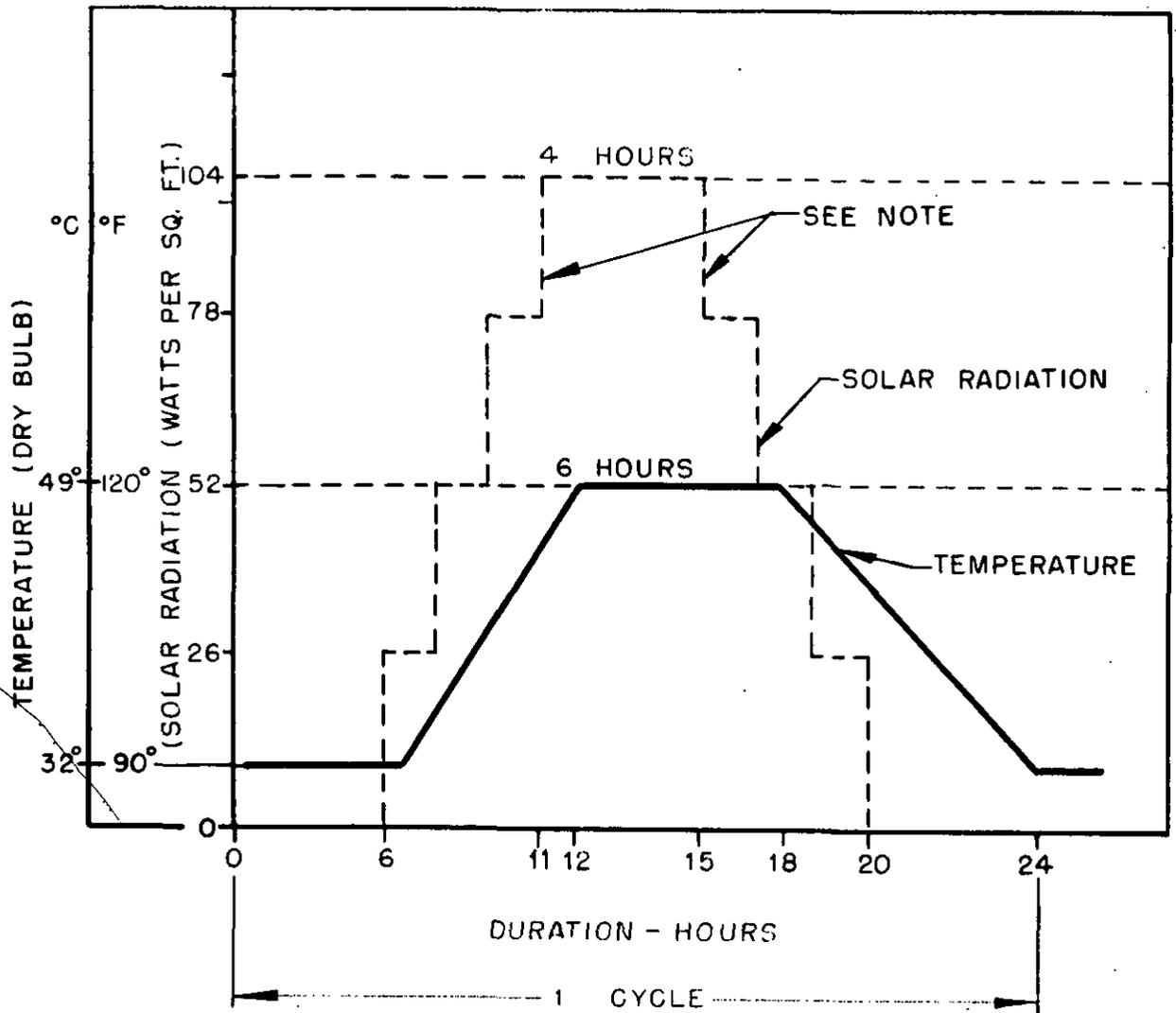
Figure 505.1-1. Accelerated Solar Radiation Cycle (Procedure II)
