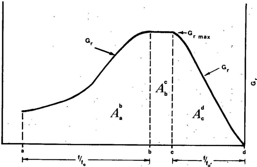
$$A_a^b = G_r \text{ max } f_0 [I_b - I_a]$$
