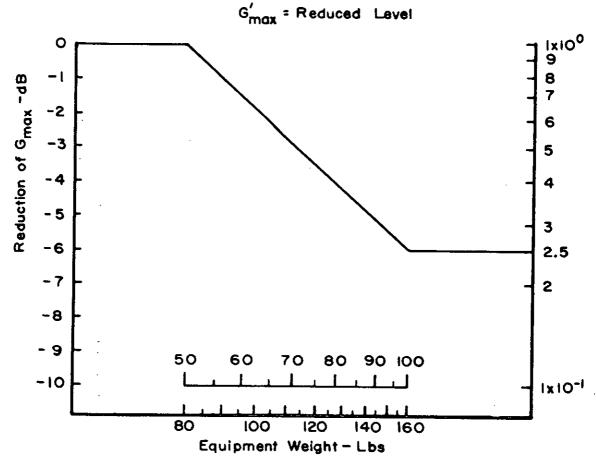
FIGURE 519.1-2. Reduction Factor for Mass Loading
