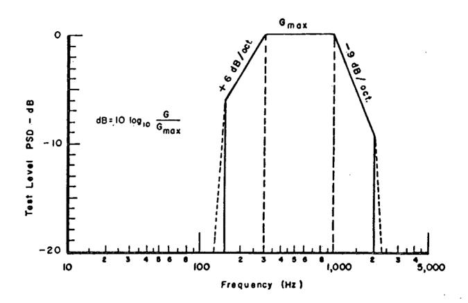
FIGURE 519.1-5. Random Vibration Test Curve
