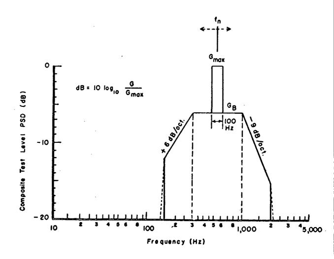
FIGURE 519.1-7. Swept Random Vibration Test Curve
