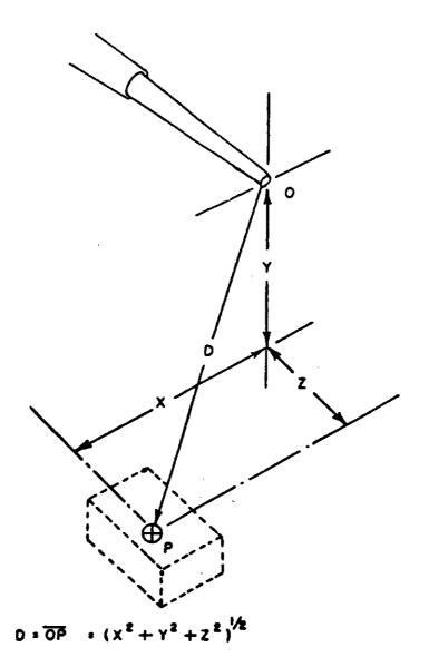
FIGURE 519.1-3. Determination of the D Vector
