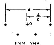
FIGURE 519.1-4. Origin of the D Vector for Multigum, Staggered Array
