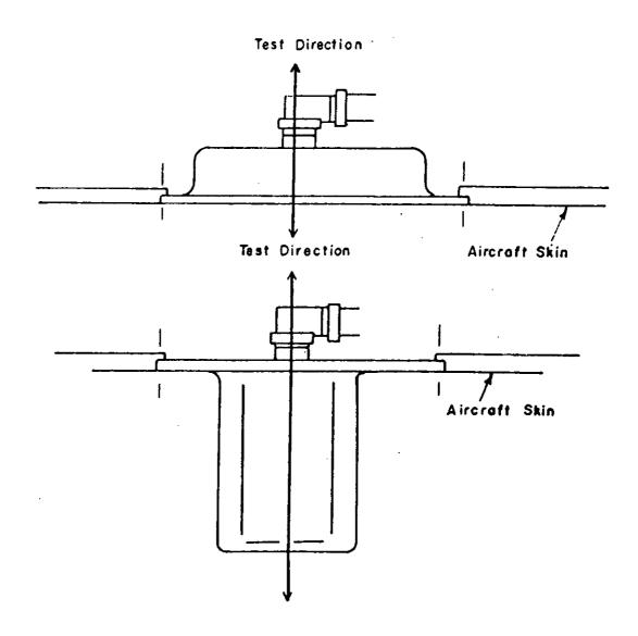
FIGURE 519.1-6. Peripherally Mounted Item
