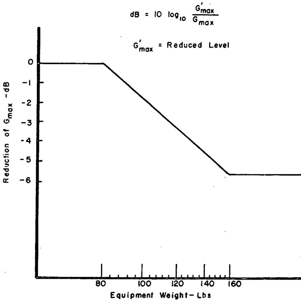
FIGURE 519-2. Reduction Factor for Mass Loading
