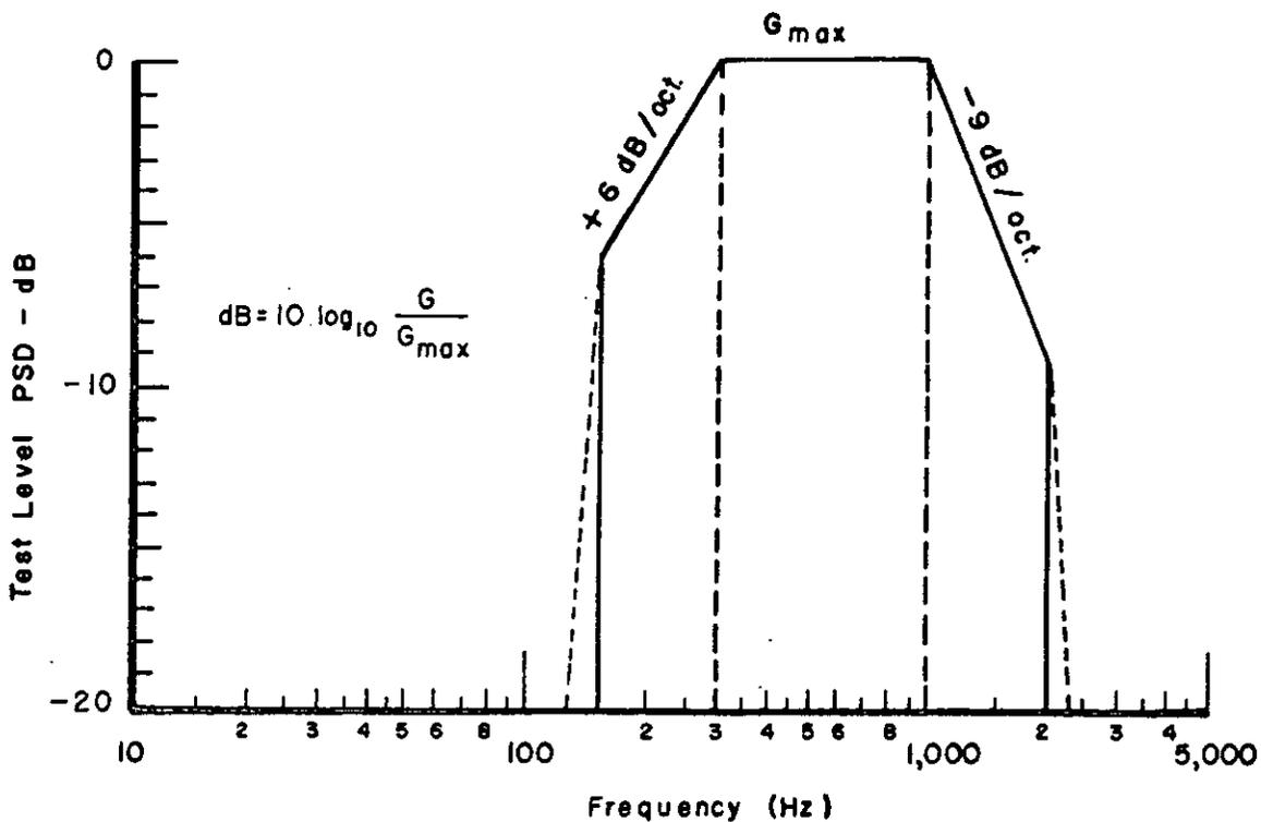
FIGURE 519-5. Random Vibration Test Curve
