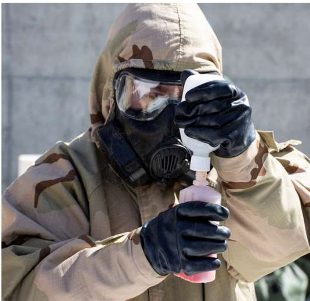
A Soldier from the 365th Chemical Company BIDS, 76th Operational Response Command, mixes the Agent Disclosure Spray, comprised of a proprietary powder and water. When sprayed on simulated or actual chemical agent, the spray changes color. Six U.S. Army Reservists and two Alabama National Guardsmen participated in the user demonstration April 20, 2021. Photos by Al Vogel, Dugway Public Affairs
