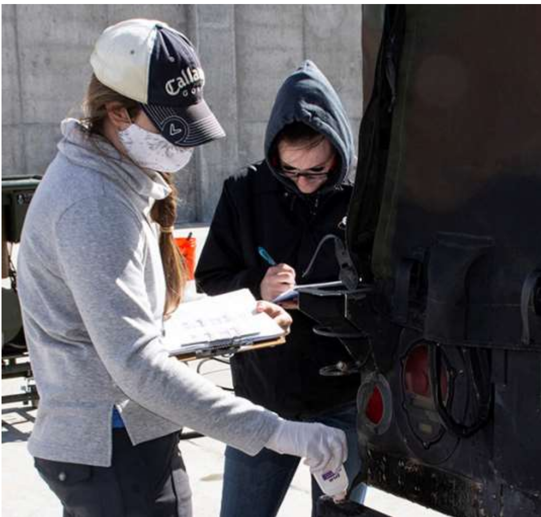
Test personnel apply a simulated chemical agent to a small spot on a vehicle April 20, 2021, so Soldiers may use the Contamination Indicator Decontamination Assurance System spray to reveal it later.
