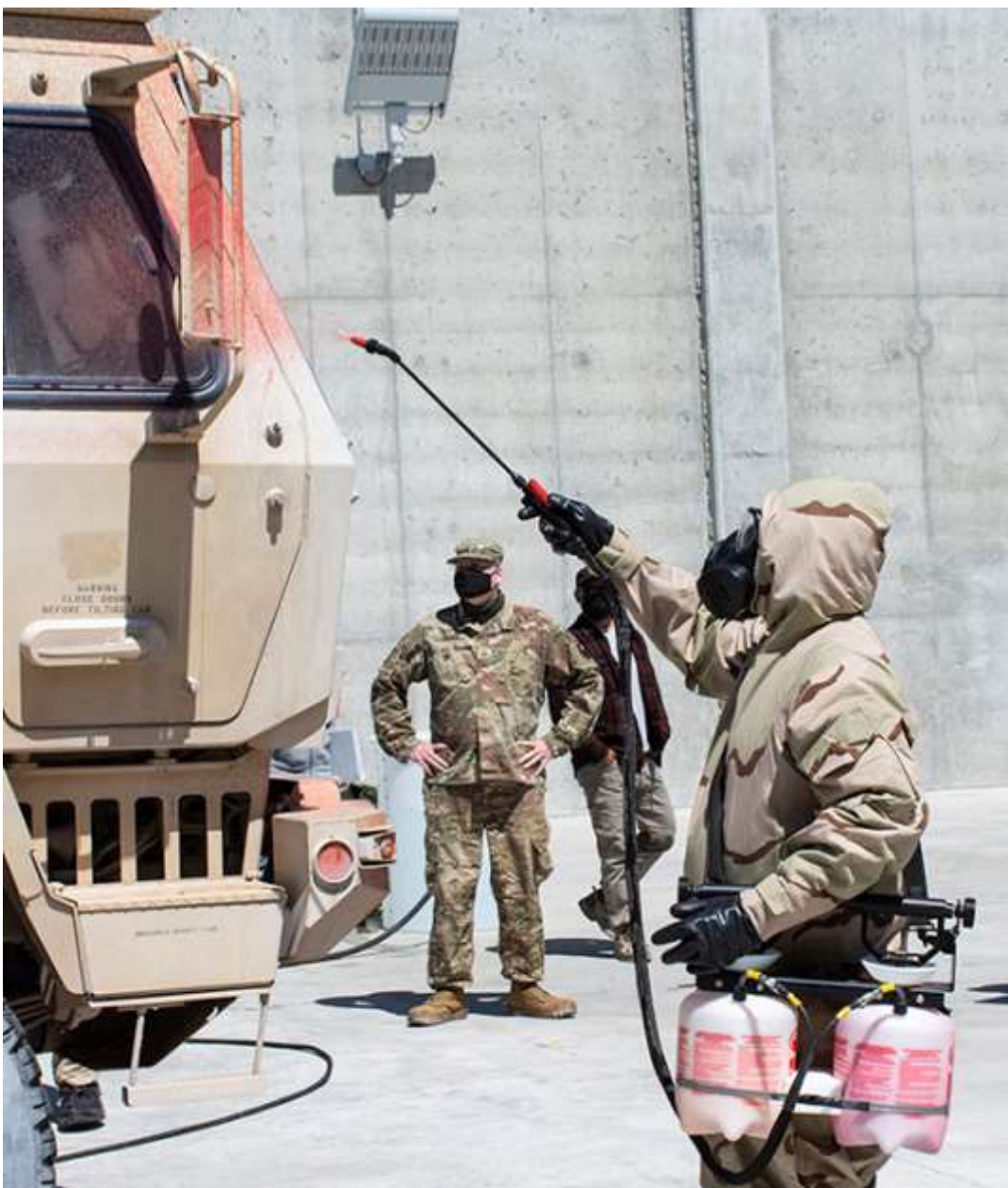
A Soldier from the 365th Chemical Company, 76th ORC sprays down a truck exterior to determine the presence of a simulated chemical agent during testing of the Contamination Indicator Decontamination Assurance System (CIDAS). The liquid turns a different color when encountering a simulated or actual chemical agent.
