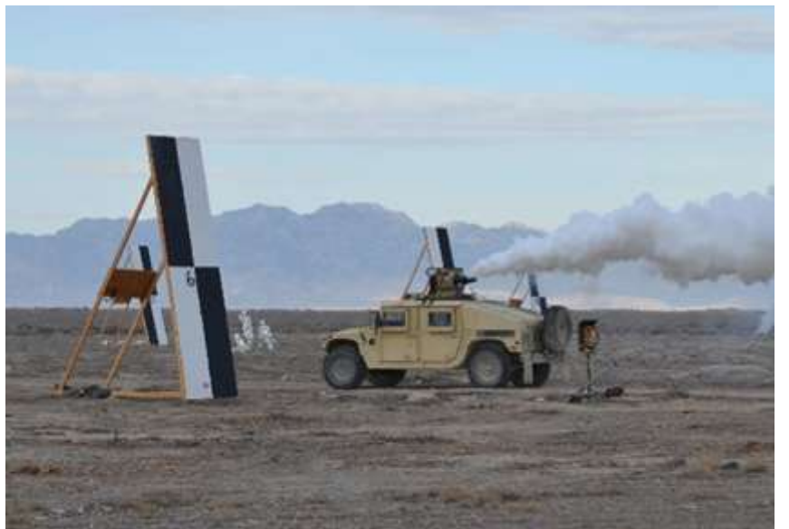
A Screening Obscuration Module (SOM) sits atop a Humvee at the start of a test trial at West Desert Test Center, Dugway Proving Ground. The mounted test trials, including cloud characterization, will continue through April. Photos by Becki Bryant, Public Affairs Office
