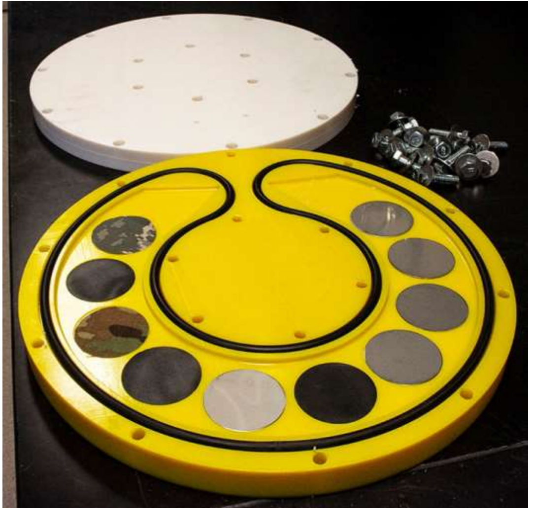
The prototype Vapor Box created by 3D printing, containing 10 fabric swatches of different material. After the white top is bolted to the yellow bottom, chemical agent is introduced through a hole at the top, and exits via a similar hole on the other side of the "horseshoe," at the top. The swatches are then removed and placed in sealed, metal "cups" for their off-gas rate to be measured. Photo by Al Vogel, Dugway Public Affairs
