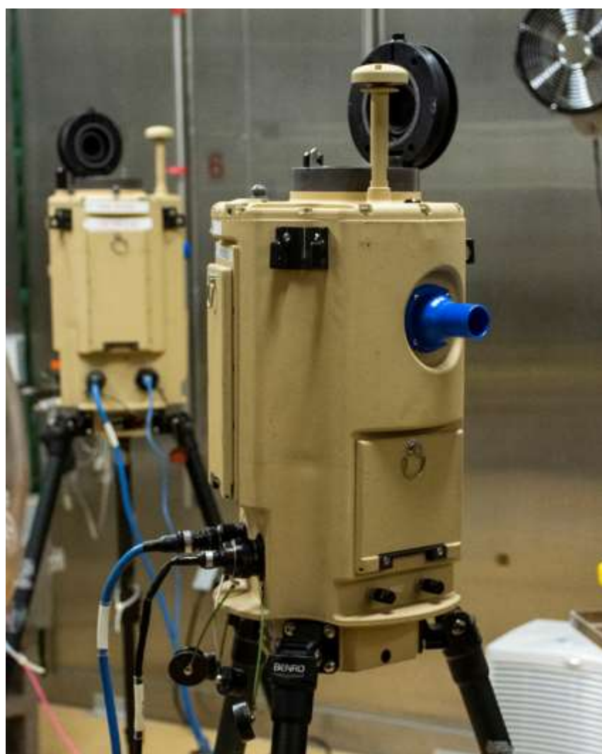
The Joint Biological Tactical Detector System (JBTDS) awaits testing with simulated agent at Dugway Proving Ground. Its legs collapse and fold alongside the detector's body, making it easier to carry and deploy than the current Joint Biological Point Detection System (JBPDS) that is larger and heavier. Photos by Al Vogel, Dugway Public Affairs
