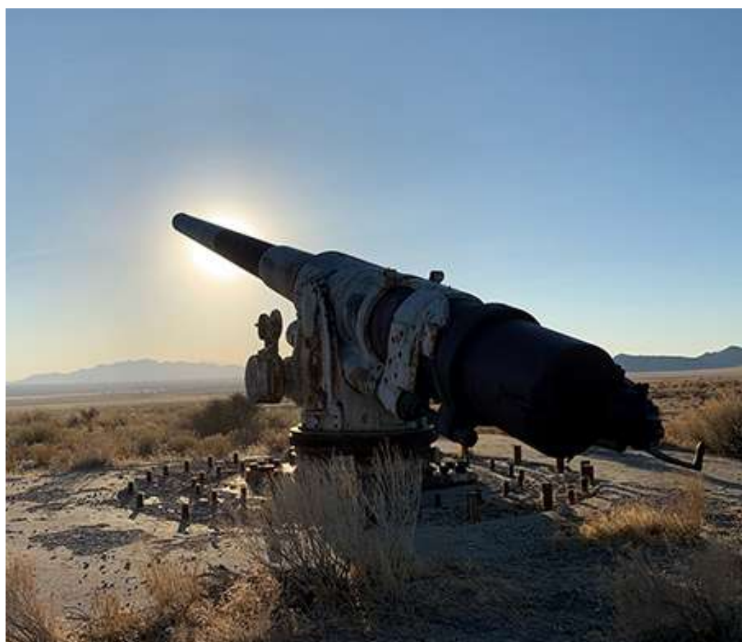
Model 1, made in 1909 at the Naval Shipyards of Washington, D.C. was brought to Dugway Proving Ground in 1955. This gun was once used to fire 6-inch diameter projectiles containing chemical agent.
