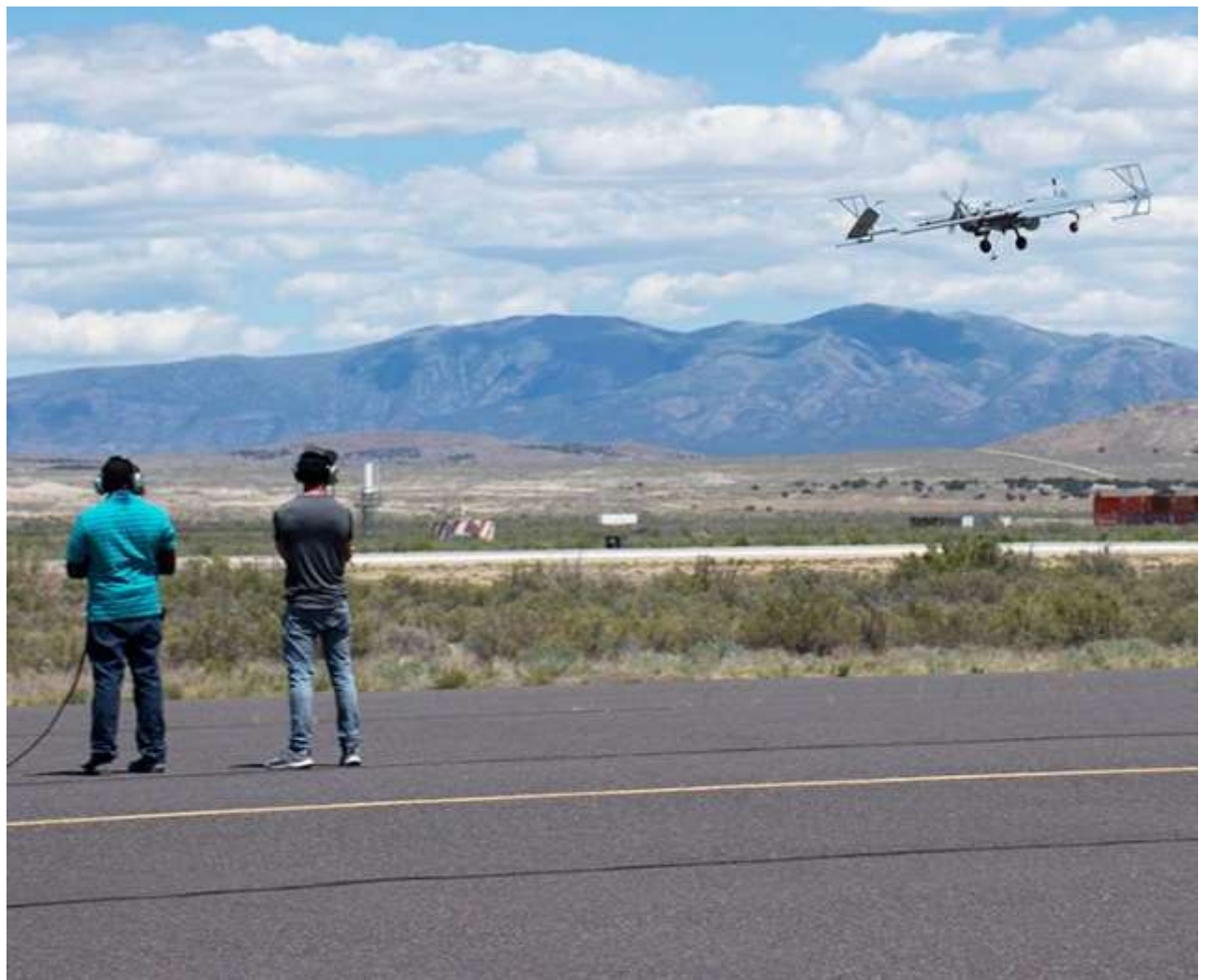
A Shadow UAS is launched from Dugway Proving Ground's Michael Army Airfield. Testing of the system's upgrades was recently done remotely. Remote testing eliminates the need for many of the test personnel to travel to Dugway. Photo by Al Vogel, Dugway Public Affairs
