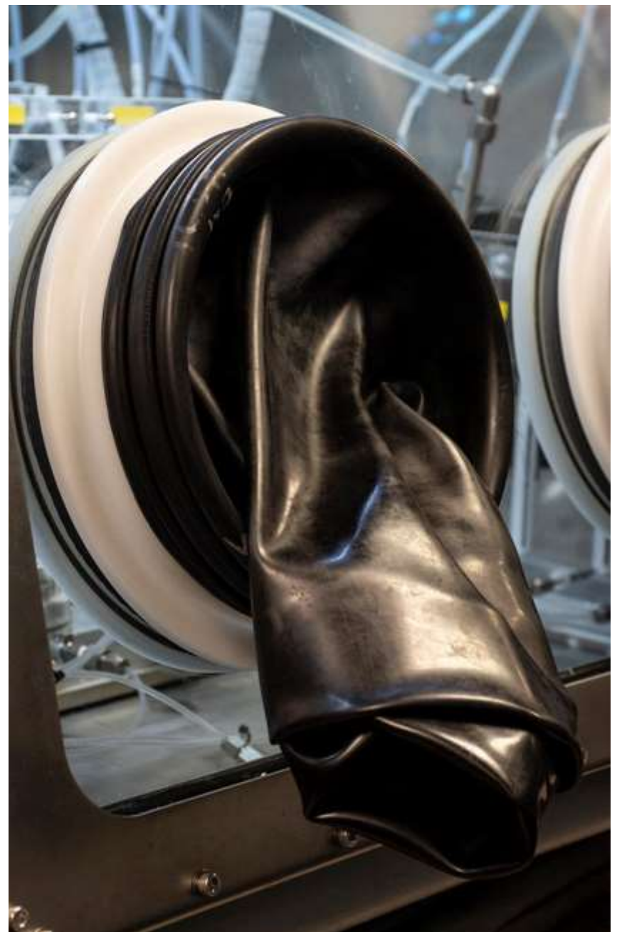
Material from a new lot of glovebox gloves, similar to this one, is being tested to determine if the gloves can resist agent breakthrough long enough for safe use within the Chemical Test Division. At the same time, SPITFIRE is using the glove testing to verify and validate that the test fixture itself functions as designed and is accurate. This classic example of downing two birds with one stone saves time and money, and reduces waiting time for the next customer.
