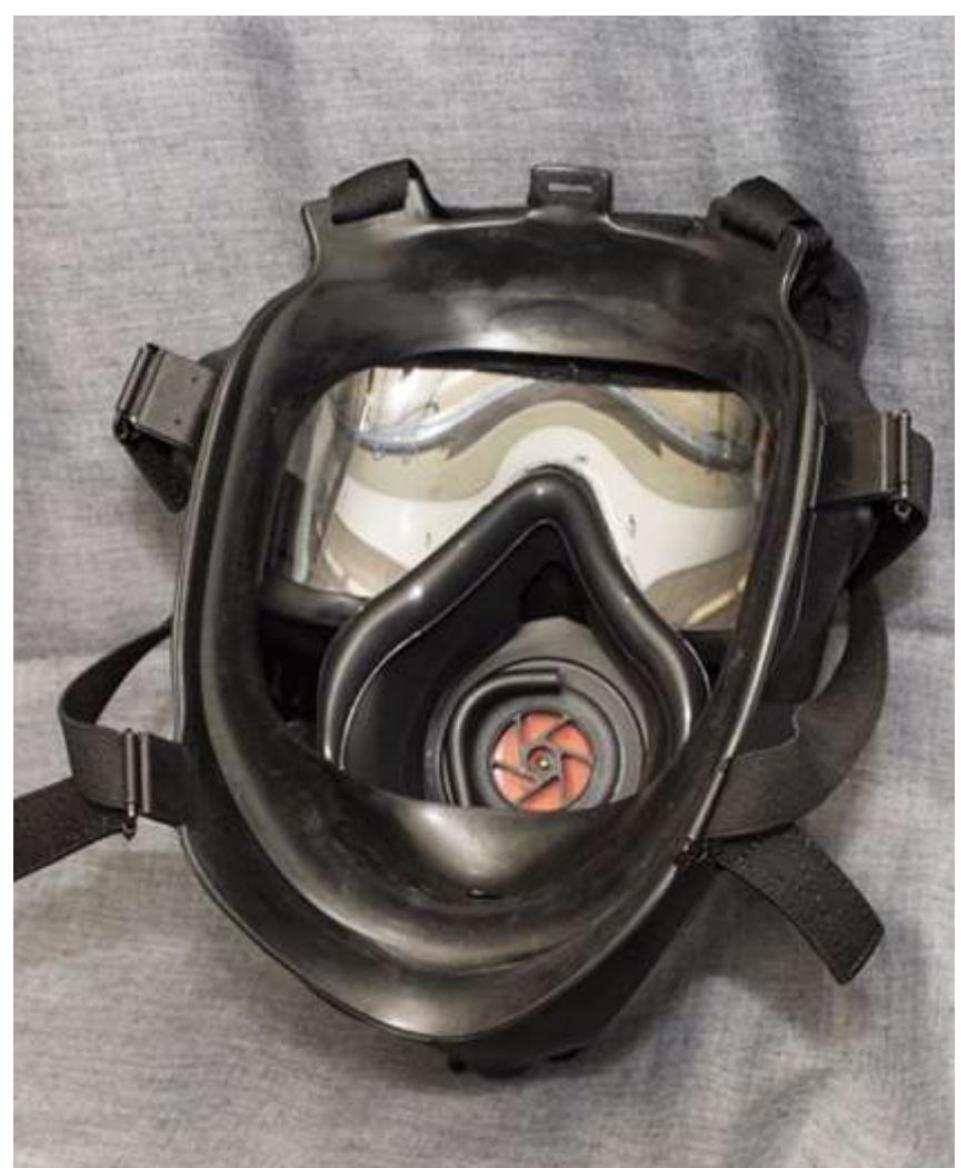
A new reflex seal inside the M53 mask provides high levels of protection and comfort to the wearer. Inside, there is also a high-flow tube that may be attached to bladders or canteens, for drinking water without removing the mask. The flexible panoramic lens minimizes visual stress and maximizes field of view.
