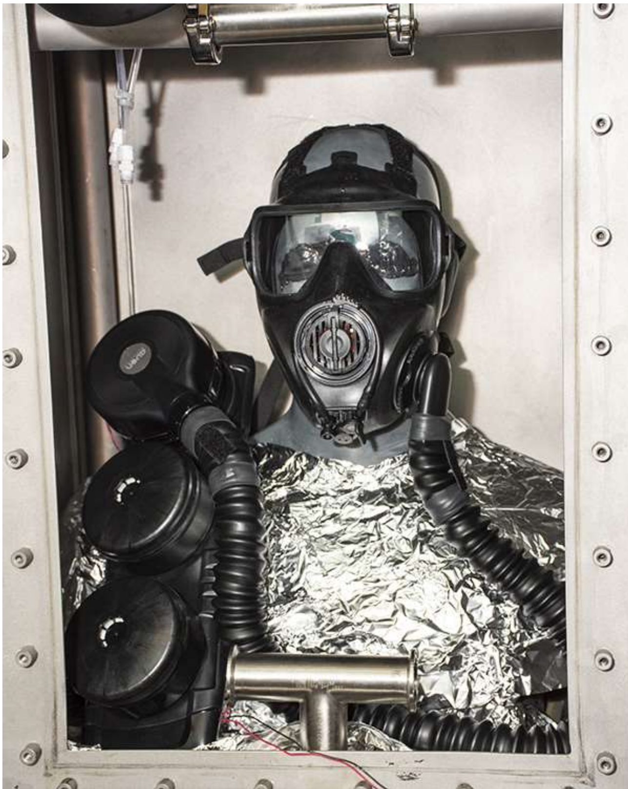
The M53 protective mask was developed to counter multiple threats found on the modern battlefield, war on terrorism and response by Special Operations units. Dugway Proving Ground recently received M53 masks for extensive testing. Here, one is attached to the Simulant Agent Resistance Test Manikin (SMARTMAN) fixture that simulates breathing patterns. Across the manikin's chest is a Powered Air Purifying Respirator that reduces breathing resistance by supplying filtered air to the mask. Photos by Al Vogel, Dugway Public Affairs
