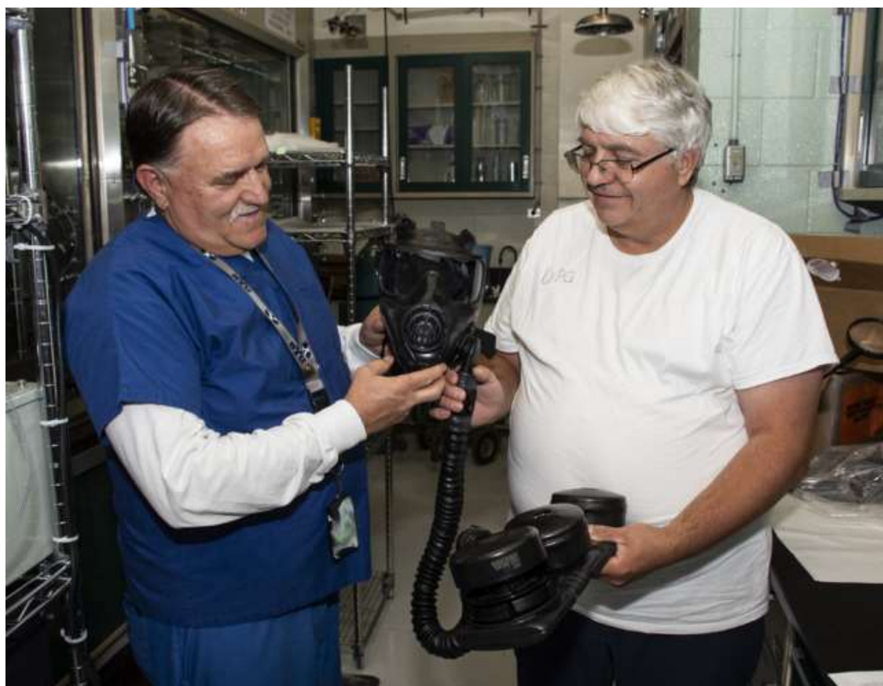
David Rose, project scientist for the M53 test (left) looks over the protective mask with Jim Haines, senior analyst. The M53 is based on the U.S. Government M50 Joint Services General Purpose Mask that replaced the M40 mask across all services. The M53 is designed to work with most PPE (Personal Protective Equipment) without having to remove or change components. It can supply its wearer with filtered air from surroundings, tanks, air purifying respirator or rebreather.
