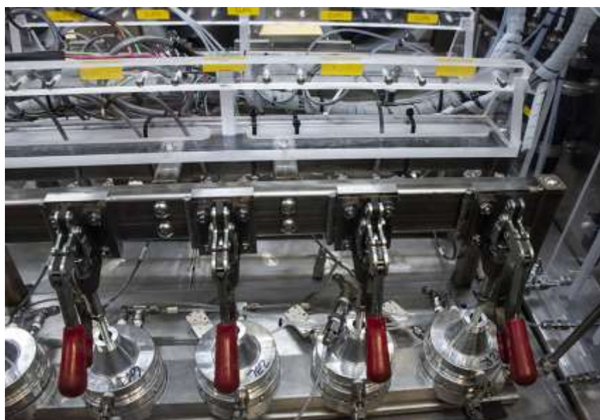
SPITFIRE (Swatch Permeation Test Fixture, Reengineered) is a swatch testing fixture more easily set up than the AVLAG (Aerosol Vapor Liquid Assessment Group) created more than 20 years ago.
