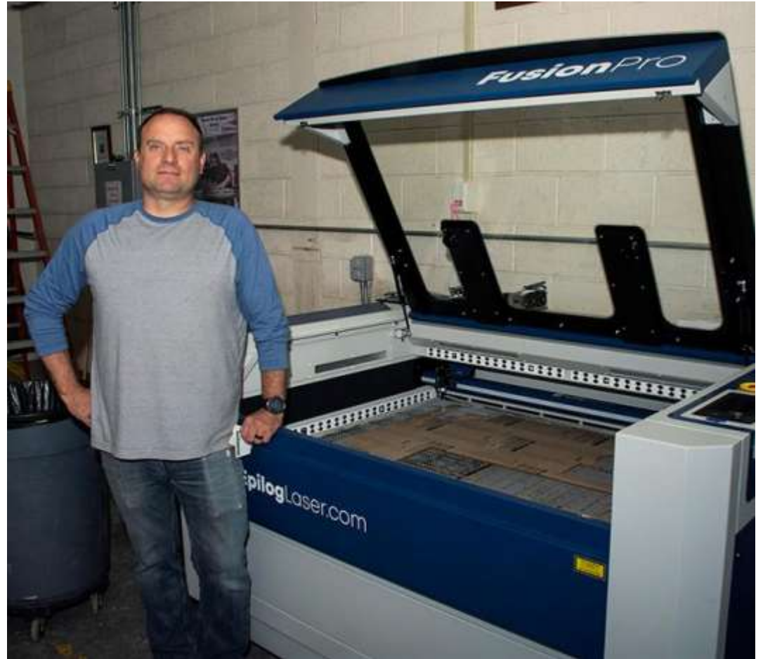
Jody Nielson, an Engineer Technician with the DPG Metal Shop, stands beside a computerized laser cutter used for cutting acrylic sheets. It cuts to exacting dimensions, and the pieces require no smoothing or final finishing, saving a lot of labor, time and expense. Photos by Al Vogel, Dugway Public Affairs
