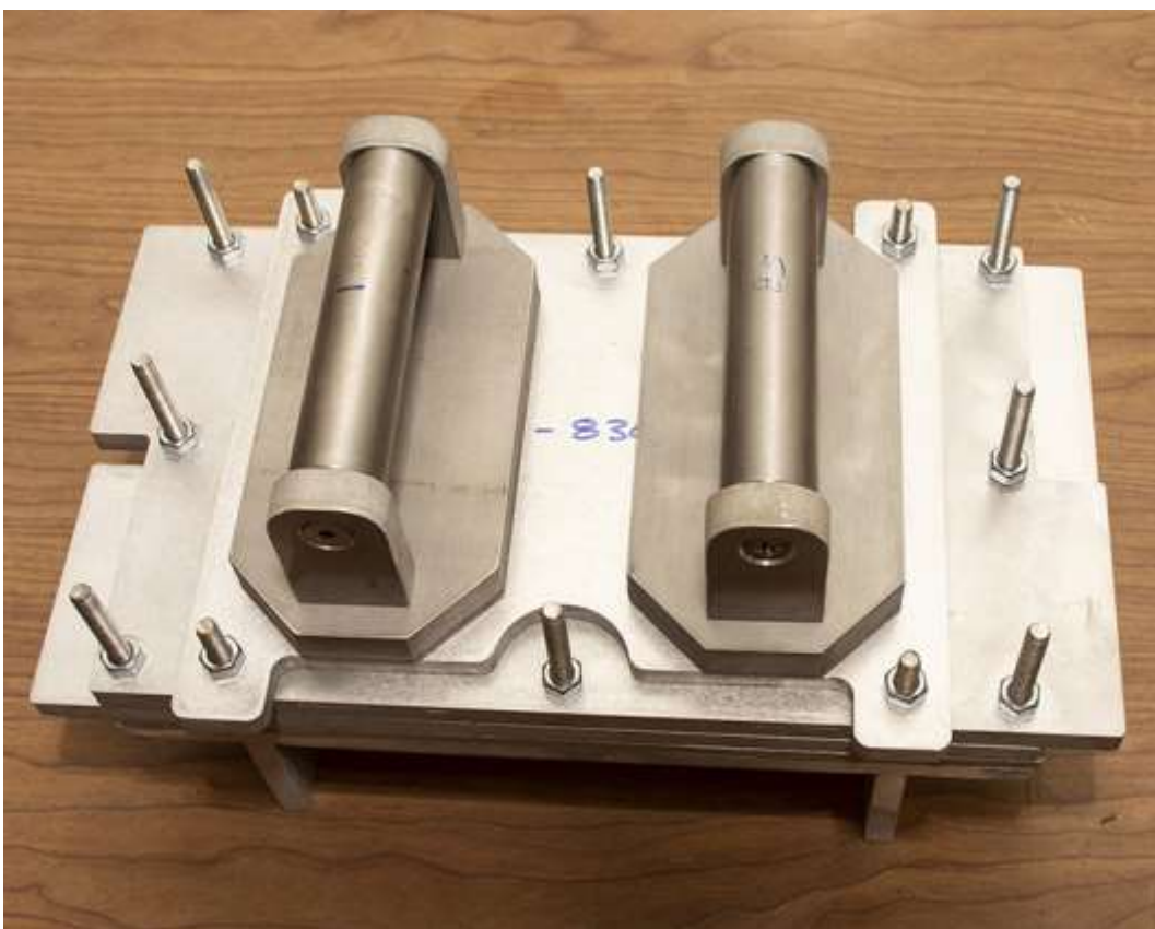
The completed test cell, as it would appear during testing in a fixture. The agent-contaminated material with a bulky closure such as a seam or zipper is held securely between two plates, called "tracks."
