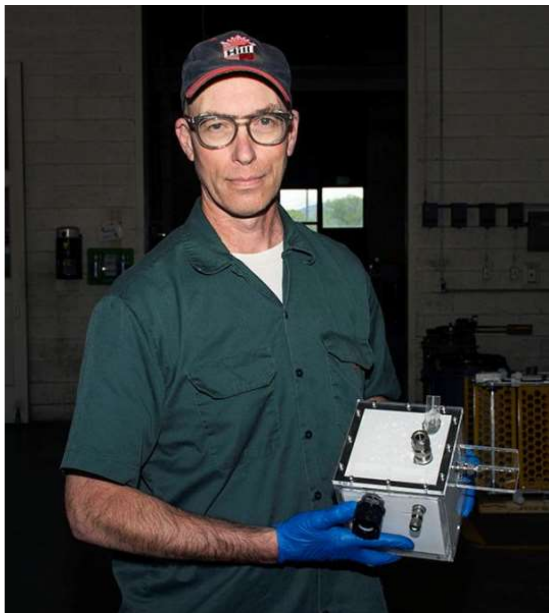
Sam Hill, DPG Metal Shop Supervisor, holds a Secondary Containment Box his shop crafted largely from acrylic. The box will contain a sensor to count the number and size of chemical vapor droplets passing through—important data when testing chemical agent detectors.
