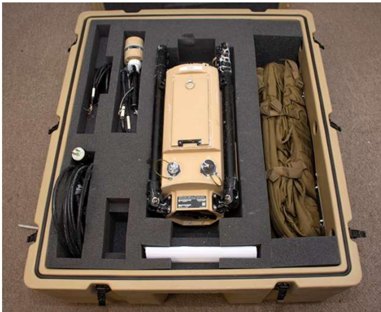
The Joint Biological Tactical Detection System is man-portable and battery powered. Transported by sea, air or land, it must function in a variety of environments. Its carrying case faces the same challenges, and is rigidly tested to ensure it will protect the detector that warns of a biological agent presence. Photo by Al Vogel, Dugway Public Affairs
