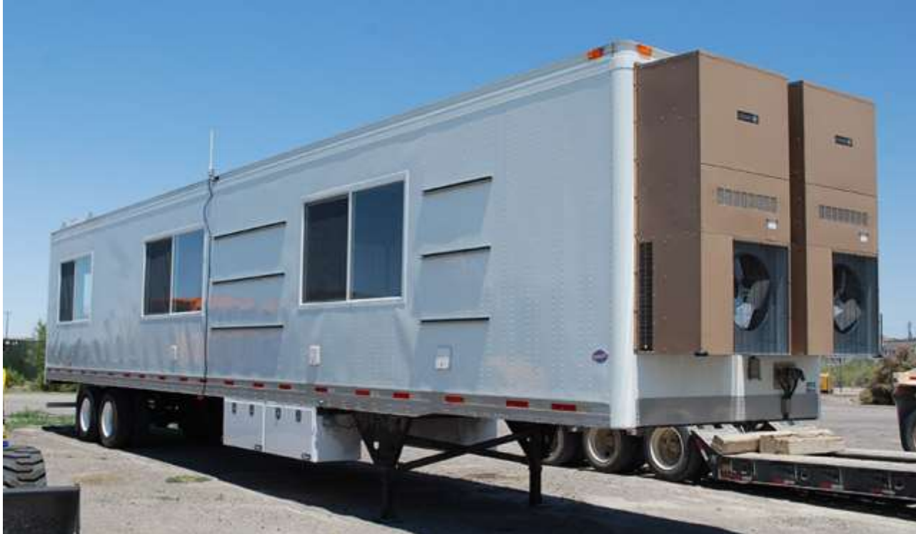
Dugway Proving Ground took receipt in December 2019 of a mobile, faster data system for testing chemical and biological agent detectors outdoors, using simulated agent. This Relocatable Command Post is part of the Test Grid Safari Instrumentation System. Photo by Joe Mashinski, U.S. Army
