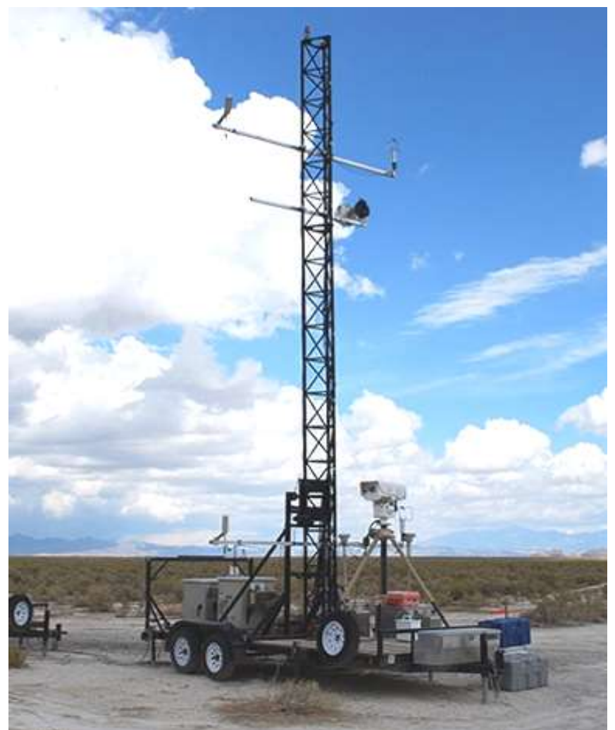
A mobile, 10-meter instrumentation tower is ready for testing on Dugway Proving Ground. Each trailer holds an electrical generator, data storage and communications. An inexpensive tent protects supplies and tools from the weather. U.S. Army photo
