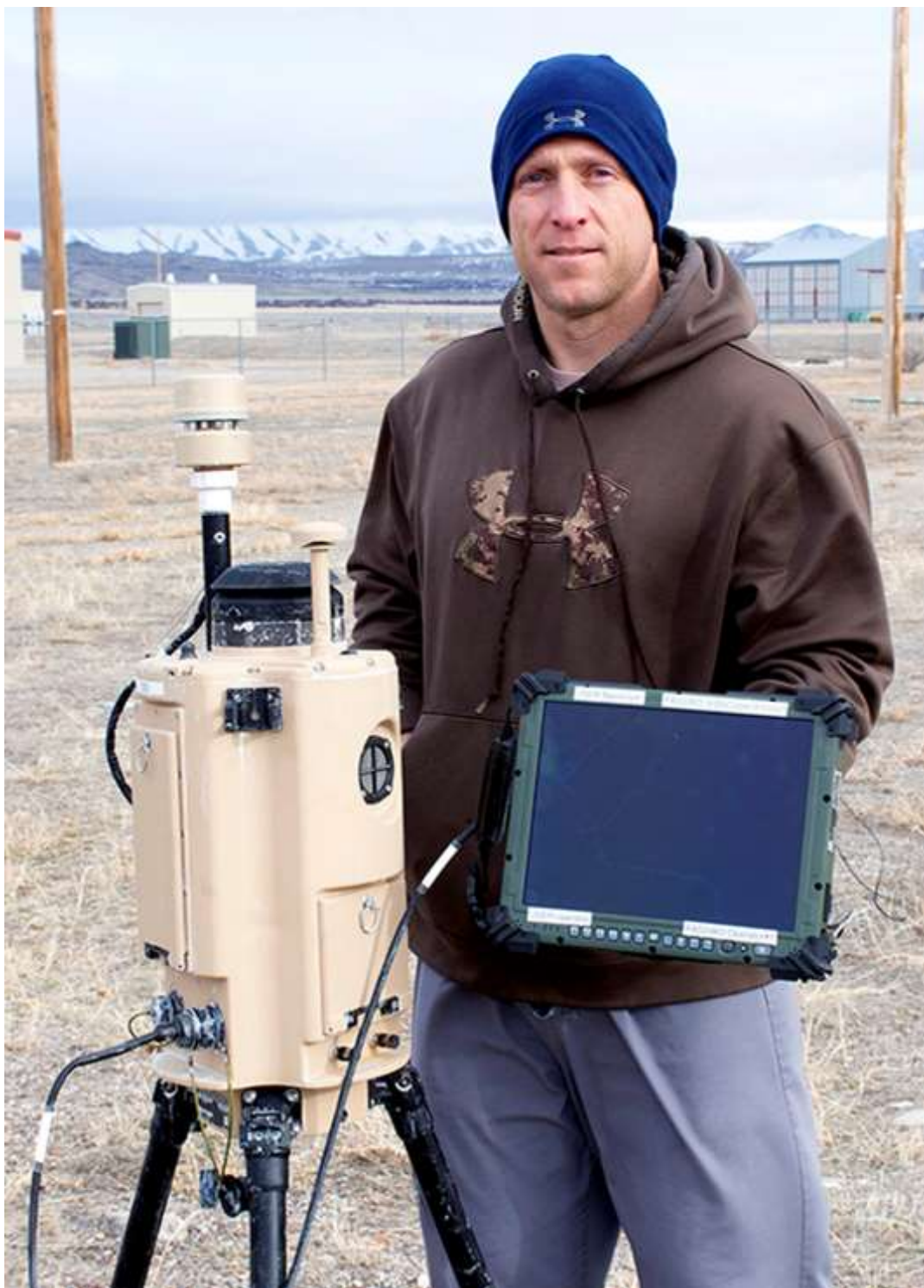
Test Director Jon Hogan stands beside a Joint Biological Tactical Detection System (JBTDS) after a salt fog environmental test at Dugway Proving Ground. Hogan holds the JBTDS base station, which can control one unit, or a number of them for perimeter defense. Photo by Al Vogel, Dugway Public Affairs
