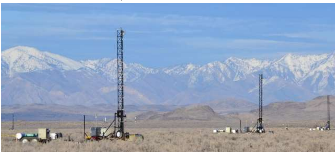
Several 10-meter towers are raised in place with instrumentation affixed, ready to test chemical or biological detectors with simulated agent. The portable towers are part of the Test Grid Safari Instrumentation system, which was recently turned over to Dugway Proving Ground. U.S. Army photo
