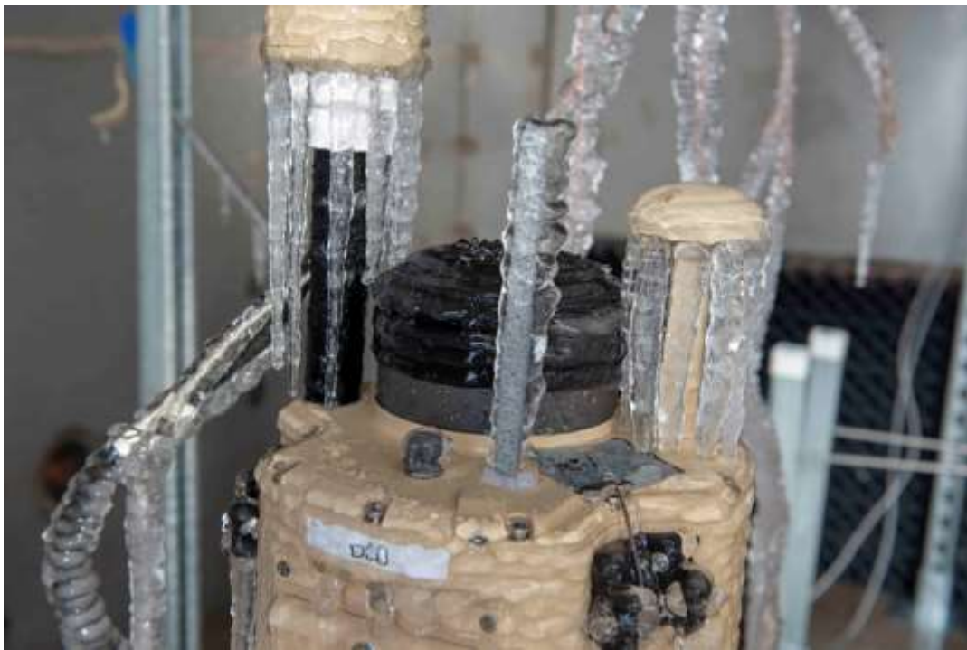
The integrated detector and collector of the Joint Biological Tactical Detection System (JBTDS) must function, and not be damaged, in this freezing-rain environmental test. Photo by Brittani Yale, Dugway Scientific Technical Photographer
