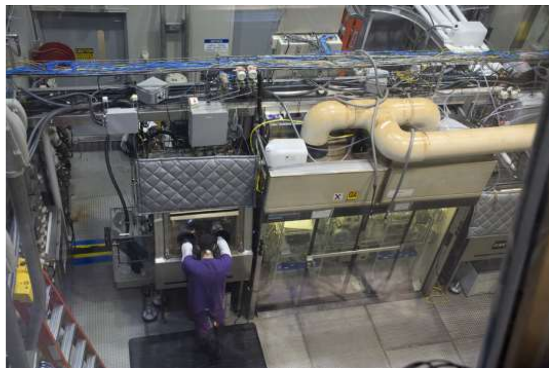
A technician uses a glovebox to make adjustments to the Chemical Agent Vapor fixture, preparing to challenge three (unseen) chemical agent detectors during developmental testing of the system. Developmental testing establishes the fixture's capabilities before scheduled testing begins. Photo by Al Vogel, Dugway Public Affairs
