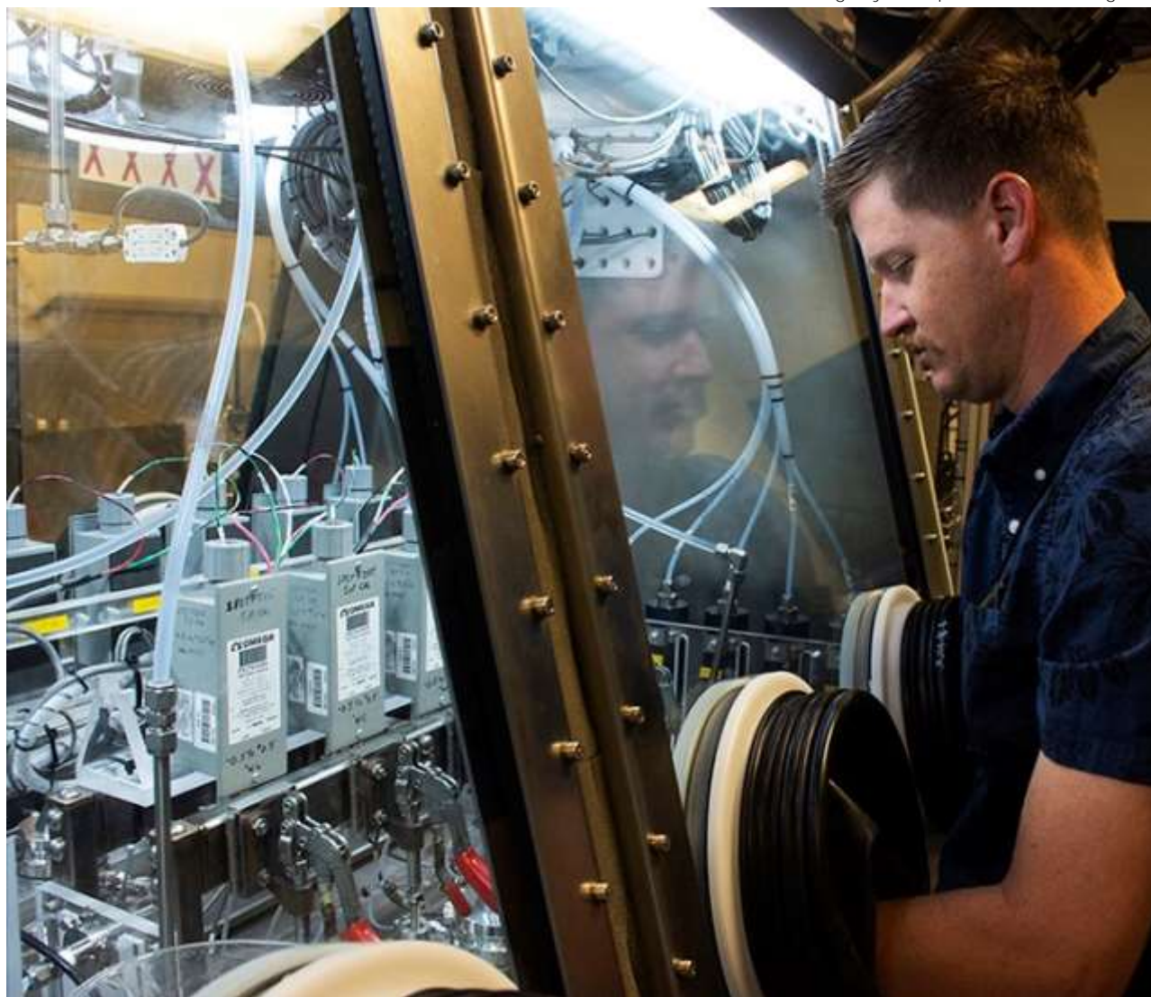
Aaron Rogers, project scientist at Dugway Proving Ground's Chemical Test Division, works with the newly created Swatch Permeation Test Fixture, Reengineered (SPITFIRE). Material considered for protection against chemical warfare agents, in the form of gloves, clothing, boots, etc. is challenged with chemical agent in this glovebox to learn how well it protects and whether it degrades. Photo by Al Vogel, Dugway Public Affairs
