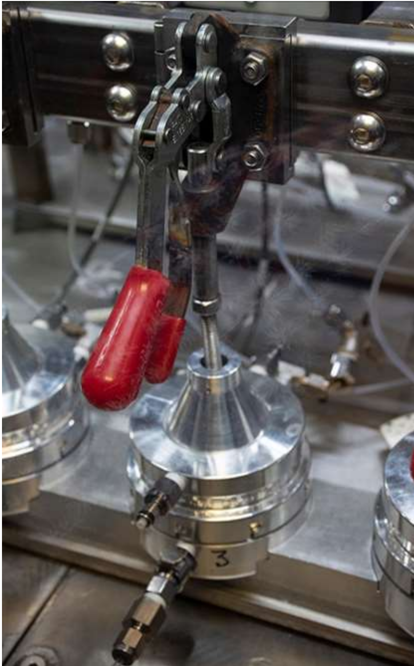
The Swatch Permeation Test Fixture, Reengineered (SPITFIRE) employs clamps to keep the components under pressure and together, instead of bolts. The newly created system challenges swatches of cloth with chemical warfare agent inside the stainless steel cup, to determine how effectively the material will protect service members from chemical exposure. Photo by Al Vogel, Dugway Public Affairs
