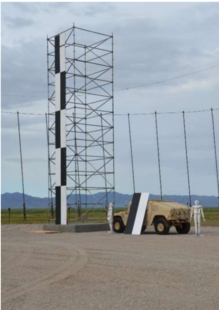
Data points were marked by a number of targets including black-and-white boards, mannequins and combat vehicles. The scaffold towers were built specifically for the SOM testing. While the scaffolding will be removed, all but one of the concrete pads will remain in place. Photo by Becki Bryant, Dugway Proving Ground Public Affairs
