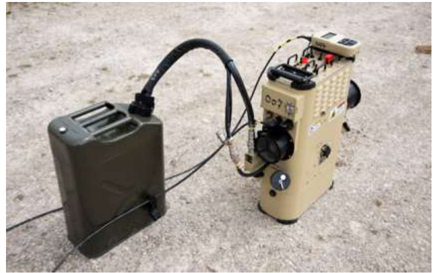
The SOM is a portable, remote-controlled obscurant generator that can be operated while mounted on a combat vehicle or dismounted (as shown in picture above). The SOM is sized so that it fits in a standard dual fuel can holder. The generator unit is paired with a 5 gallon capacity prepackaged obscurant reservoir containing SGF2. Photo by Sarah R. Densing, Scientific Technical Photographer, Dugway Proving Ground
