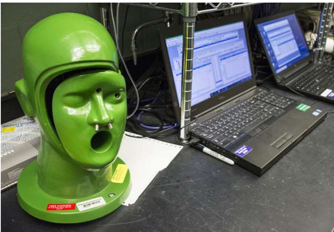
The newer version of a SMARTMAN fixture, with a specialized coating to replicate the natural compressibility of human skin. Tubing in the head draws air through the nostrils and mouth, which is constantly monitored. SMARTMAN testing creates a wealth of data, recorded and archived for later research. Photo by Al Vogel, Dugway Proving Ground Public Affairs
