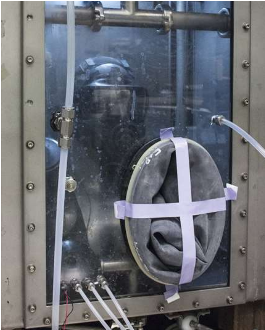
The M53A1 mask differs from the original M50 to allow prone shooting, use with aircraft oxygen systems, breathing apparatus in an enclosed protective suit and NATO-standard filters. Photo by Al Vogel, Dugway Proving Ground Public Affairs
