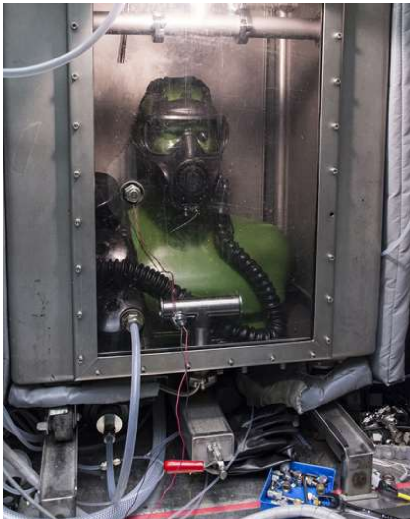
The M53A1 protective mask, a variant of the current issue M50. This version has been altered for use by aircrew, for direct feed from the aircraft's oxygen supply. The M50 protective mask has been tested at Dugway Proving Ground since 2001, and was first issued to all services in 2009. It is not uncommon to alter a mask for special applications, requiring additional testing. Photo by Al Vogel, Dugway Proving Ground Public Affairs
