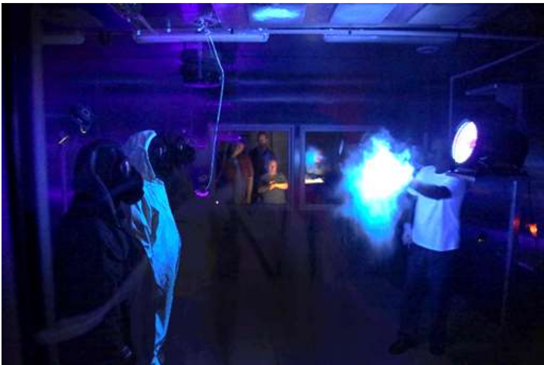
BioTesting Division Microbiologist Scott Jonas activates a party popper filled with Glo Germ dust within the Aerosol Simulant Exposure Chamber as three Soldiers from the Alabama National Guard's 690th CBRN Company wait in protective suits for the dust to disperse. Photo by Jack Bunja
