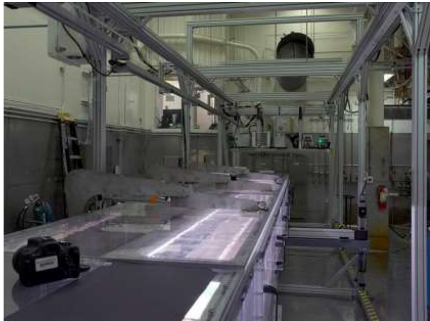
The detector rides on an overhead track, replicating its use on reconnaissance vehicle, and is challenged to visually detect chemical agent on dirt, concrete, asphalt and other sample surfaces inside the 30-foot chamber. Rectangular openings in the top of the chamber allow the detector to view directly below, without interference from plastic or glass walls. Chemical agent is kept from escaping the chamber by strong air suction and filtration. Photos by Al Vogel, Dugway Public Affairs
