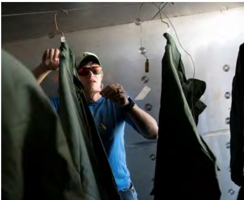
AJ Line, an engineering technician with the West Desert Test Center, prepares to move Warfighter suits from the hot/humid chamber into the cold chamber for additional testing. Photos by Daniel Jay Bryant, Dugway Scientific Technical Photographer
