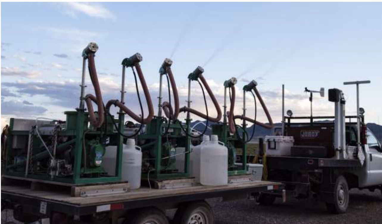
Simulated chemical or biological agents were used exclusively for the three weeks that CENTAUR was tested, and Warfighters from overseas participated in real-time scenarios to evaluate the system. Seen here are disseminators on a trailer, for easy movement in the field to place the simulated agent cloud upwind of the detectors. Some test trials include interferents such as dust and smoke, to ensure detectors are not affected by other substances in the air. Photo by Mario Sandoval/ Dugway Optics
