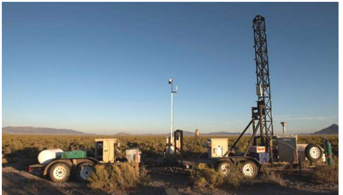
Some systems comprising the CENTAUR, in the field. An instrumentation tower supports the test, while a combination of CENTAUR detection, monitoring and communication equipment is challenged with simulated chemical biological or radiological (CBR) threats. The CENTAUR system was also tested by Soldiers challenged by real-world scenarios, requiring them to make real-time decisions based on what CENTAUR provided. Photo by Mario Sandoval / Dugway Optics
