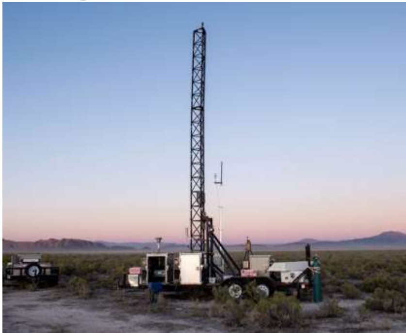
A portable instrumentation trailer, with fold-down 10-meter tower, makes setup and testing easier. CENTAUR was expected to receive 30 trials of different simulants, but 53 trials were conducted, thanks to an exceptional test crew and ideal weather conditions. Photo by Mario Sandoval/ Dugway Optics
