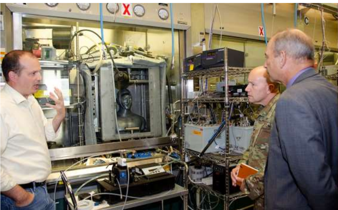
Bryan Fausett, chief of the Chemical Operations branch of Dugway Proving Ground's Chemical Test Division (left), explains how gas masks and respirators are tested on the SMARTMAN mannikin in a sealed chamber. Right: Col. David Trybula, Commander of White Sands Missile Range (WSMR) in New Mexico, and SES Richard Meador, Executive Director of WSMR, toured Dugway Sept. 25 and 26. Photo by Darrell Gray, Dugway Public Affairs
