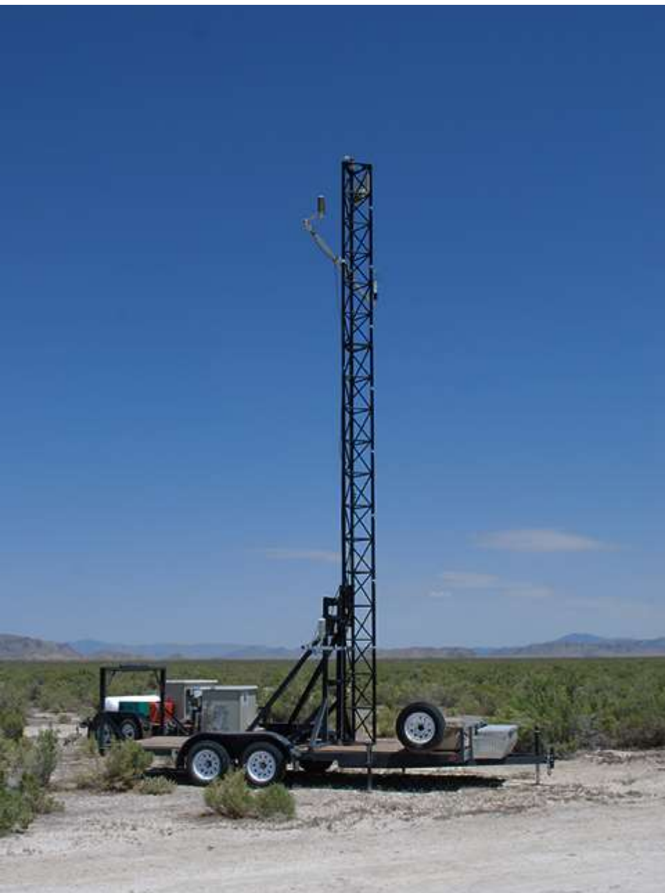
A trailer-mounted 10-meter tower, ready for its instrumentation to begin receiving data, at Dugway Proving Ground, Utah. The tower may also be folded down for travel or to work with instrumentation. The trailer also includes a Computer Network Interface for data, and a propane-fired electrical generator. A new, mobile and highly efficient system for testing chemical and biological detectors is anticipated to be complete for use this fall. Photo by Joe Mashinski, US Army
