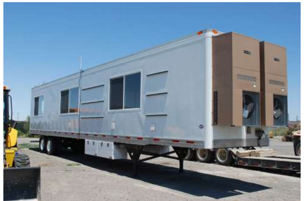
A Relocatable Command Post is part of the Test Grid Safari Instrumentation System now underway at Dugway Proving Ground, Utah. Data from testing chemical and biological agent detectors is fed into the command post after data is stored and back-up elsewhere. The mobile testing system is anticipated to be turned over to Dugway this fall. Photo by Joe Mashinski, US Army
