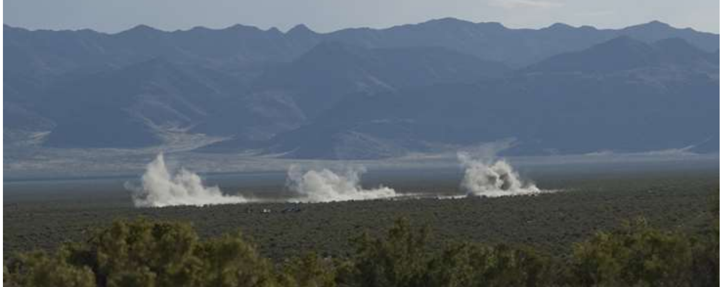
A crude but somewhat effective method terrorists might use to disseminate a chemical agent is with explosives. Here, clouds of dust and simulated agent drift toward detectors some distance away at Dugway Proving Ground, Utah. Test Grid Safari Instrumentation System, underway at Dugway and expected to be completed this fall, will test chemical and biological agent detectors with simulated agent. Photo by Al Vogel, Dugway Public Affairs
