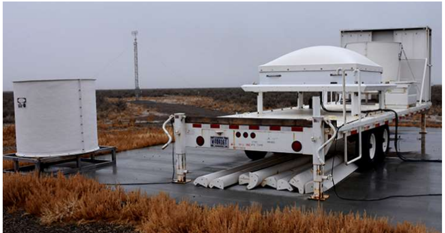
A weather radar profiler at Dugway Proving Ground scanning directly upward. The area it searches is cone-shaped, but its side profile appears on a flat monitor. The radar, in the peaked housing on the trailer, reaches up to the upper boundary layer within which most releases of a simulated chemical or biological agent take place. Photo by Al Vogel, Dugway Public Affairs
