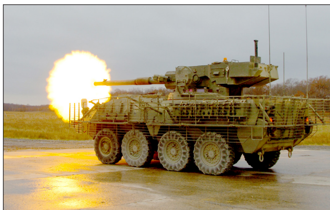
A Stryker Mobile Gun System is equipped with slat armor designed at ATC.
