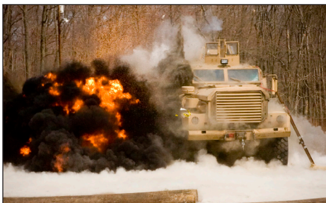
An MRAP undergoes IED-inspired survivability testing.
