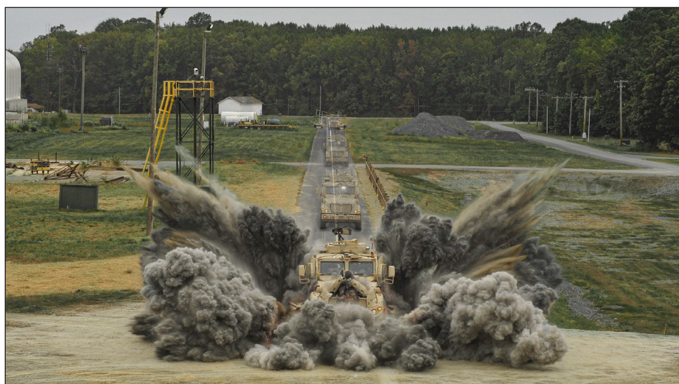
An MRAP vehicle moving at 30 mph undergoes a dynamic mine underbody blast event at ATC.
