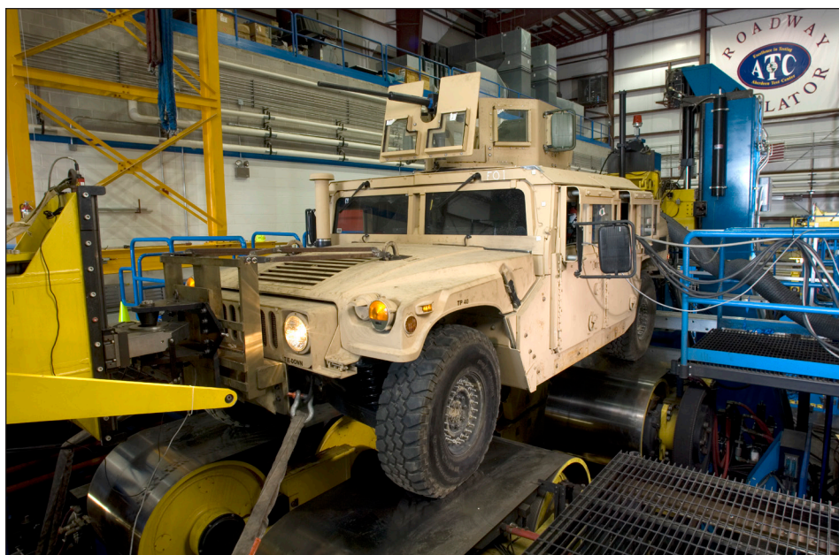
The weight of a HMMWV is no challenge to the Roadway Simulator's 13-ton capacity.
