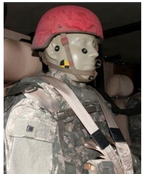
WIAMan TD participates in an MHTV Cougar test at Aberdeen Proving Ground.
