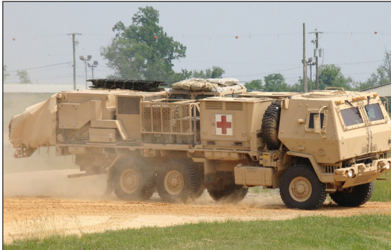
The Chemical-Biological Protective Shelter (CBPS) undergoes automotive durability testing on ATC's Munson Gravel Course.
