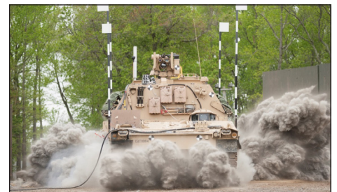
The M992A3 CAT, the M109A7 SPH counterpart, is subjected to an underbody blast.
