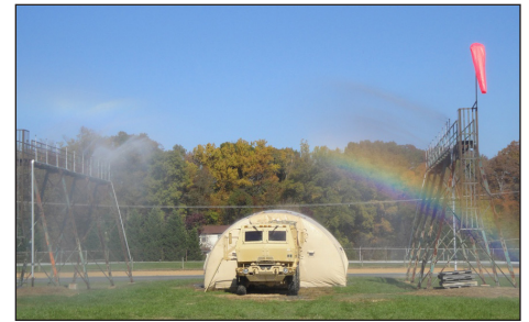
The CBPS undergoes rain testing to determine the shelter's resistance to rain infiltration.
