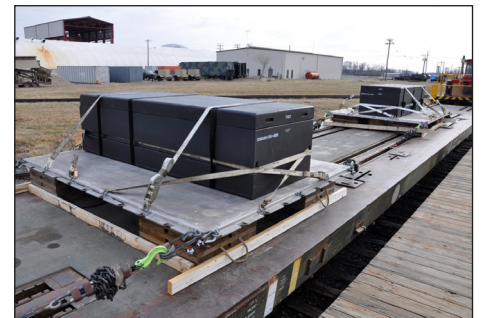
A human remains transfer system undergoes shock testing using the ATC Rail Impact Test Facility to induce test-specific shock loading.
