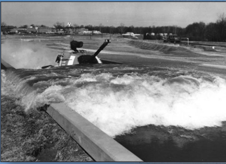
An M48 traverses the Munson Test Area Shallow Water Fording Basin, circa WWII.
