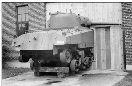
Power train efficiency test being performed on an M43 medium tank, September 1943.
