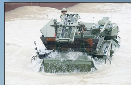
Image sequence of an Assault Amphibious Vehicle (AAV) undergoing a stabilization test in the Littoral Warfare Environment wave pond.
