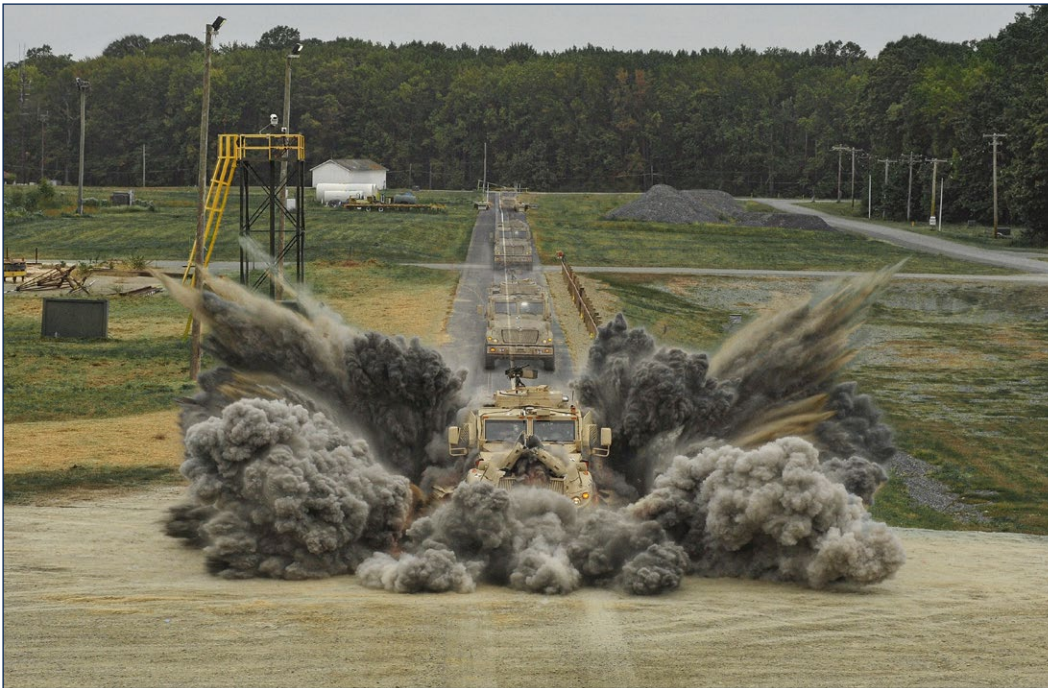
MRAP vehicle moving at 30 mph undergoes an underbody blast event at ATC.
