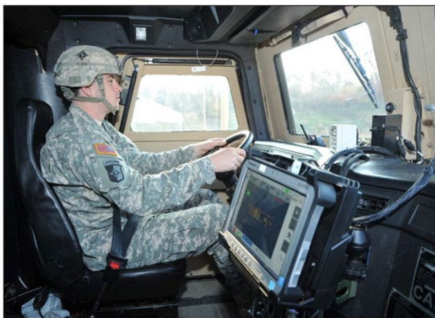
At ATEF, a Soldier operates a truck equipped with AMAS-BWASK to assess the situational awareness and active safety capabilities of the system.
