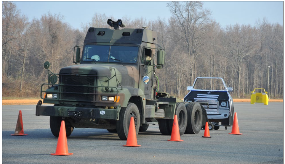
Backup plan - an Army tractor truck demonstrates the AMAS-BWASK backup-assist feature. With no driver input, the system detects the vehicle behind the tractor and applies the brakes to avoid the impending accident.
