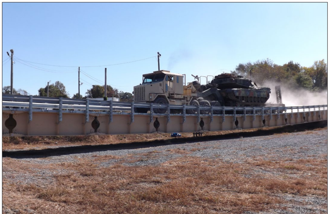
Taking the high road - a heavy equipment transporter carries the M1 Abrams battle tank, weighing almost 62 tons, across the LOCB.
