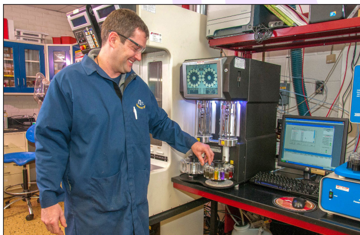
ATC chemist Mark Michie uses a kinematic viscometer and an atomic emission spectrometer to analyze oil samples in the CSAB laboratory.
